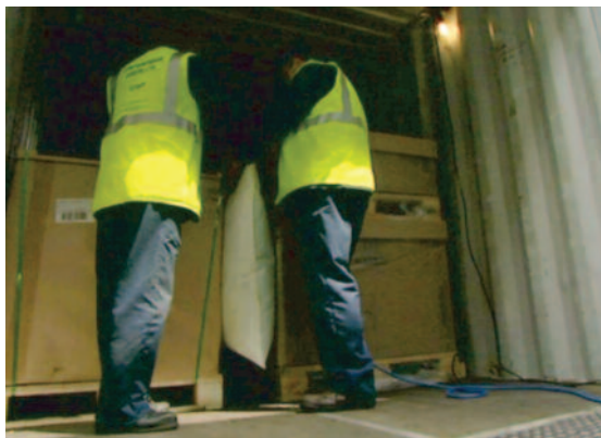
Using inflatable air bags to fill a gap between rows of pallets
