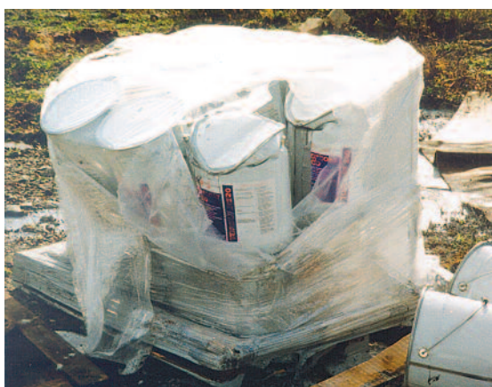
Here, a pallet has damaged the drums below. The indent of the pallet above can be seen on the top of the drum in the corner. This could have been prevented by using a spreader sheet of plywood between the tiers of pallets
