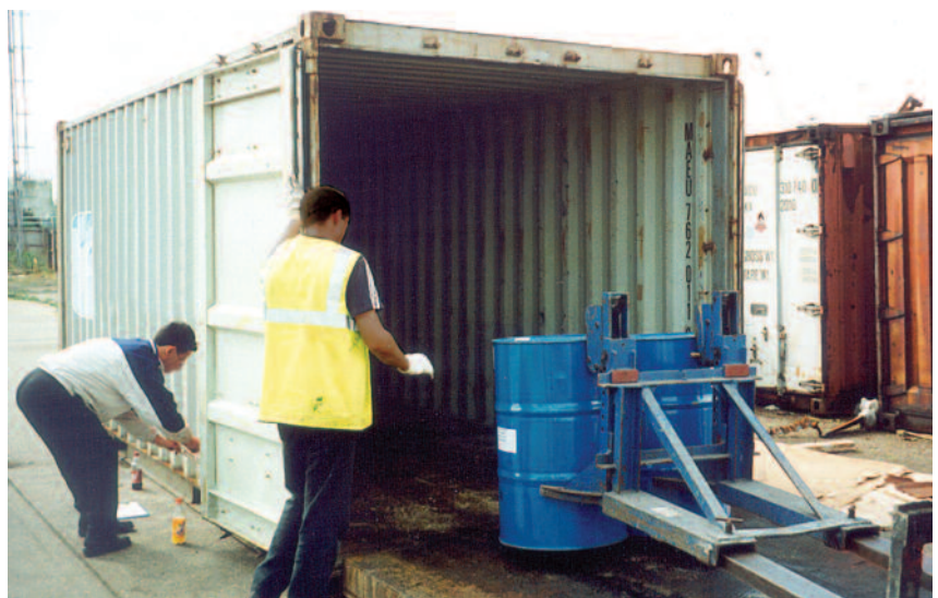
Drums being packed with drum clamps
