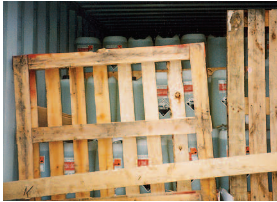
Using pallets and timber to fill a gap and make a gate between the cargo and the doors
