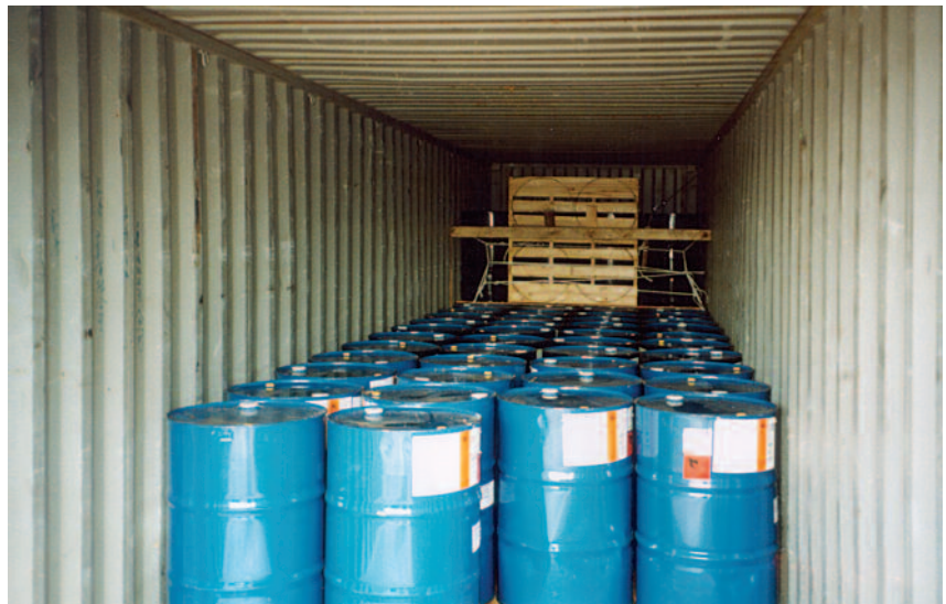
Cargo "gate" made from timber struts, rope and a pallet
