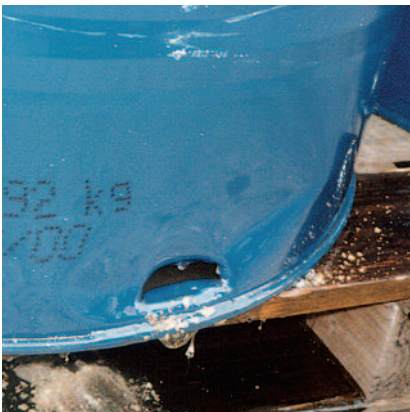
Drums stabbed by fork lift – a common cause of drum damage during handling
