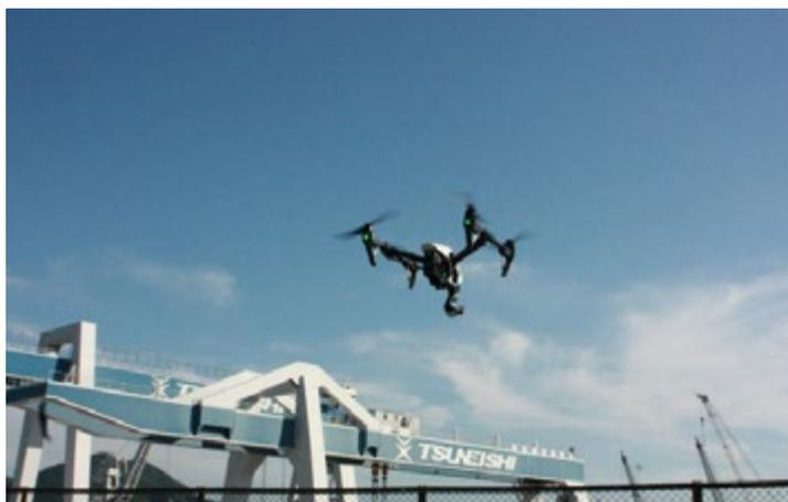
At the International Association of Classification Societies (IACS), discussions on the use of Remote Inspection Techniques (RIT) including drones in class surveys are already underway, and IACS Rec. 42 (Guidelines for Use of Remote Inspection Technics for Surveys) was revised in June of 2016. A revision of the related IACS Unified Requirements has also been completed and will take effect in January 2019.
