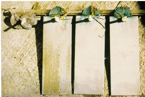
**Figure 6a.** Couples of nickel aluminium bronze discs and superduplex stainless steel plates with cathode/anode area ratio of 10:1 after 63 days in natural seawater.
