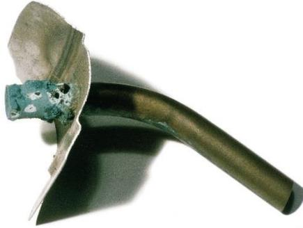
*Figure 4. Accelerated corrosion of a copper tube attached to a large stainless steel tank.*
