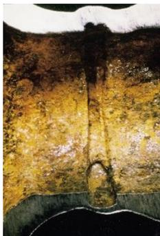
*Figure 5. Preferential corrosion of a weld in a carbon steel pipe.*
