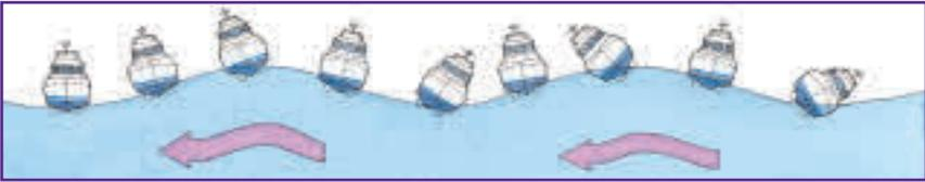
A change of heading and/or speed reduces resonant rolling motions.
