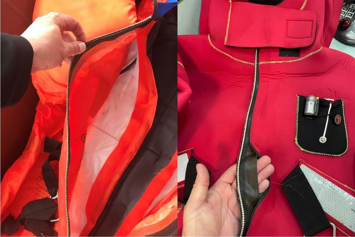
Photographs of the two aforementioned cases. Left - premature failure of zipper sealant (glue). Right - seam failed after pulling the zipper all the way up and then down. In addition to these cases, the Administrator continues to find immersion suits in unserviceable condition during Quality Control Boardings and during Annual Safety Inspections.
