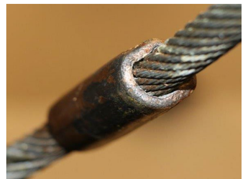
Figure 2: Completed fitting is not "round" nor within manufacturer specifications.
