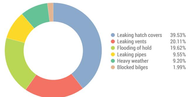
For wet damage claims, heavy weather and leaking hatch covers are both the most common and the most costly type. Indeed heavy weather and leaking hatch covers are coinciding incidents as the cargo hatch covers may be washed over by green sea on deck when the vessel sails through heavy weather.
