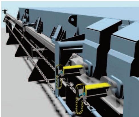
Cleats prevent the hatch cover panels from being lifted up in heavy weather. The condition of the cleats has a direct effect on the safety of the vessel. Hatch cover cleats:
