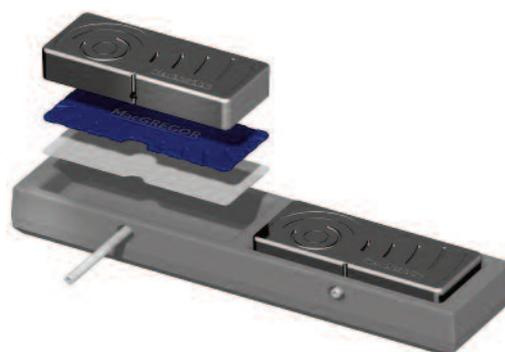
Hatch cover bearing pads transfer the weight of the cover, and any cargo it may be carrying, to the ship's hull while allowing for relative movement between the cover and the hatch coaming caused by hull flexing in a seaway. They must also maintain the correct compression on the hatch cover gasket and avoid wearing damage to the coaming/hatch cover interface.
