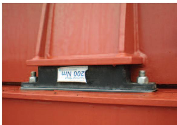
After the repair of the bearing pads the weathertightness of the hatch covers should be tested with a hose test or using ultrasonic testing equipment.
