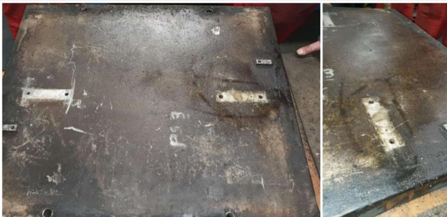
*Figure 5 - Oily substance on top of insulation panel PS3*
