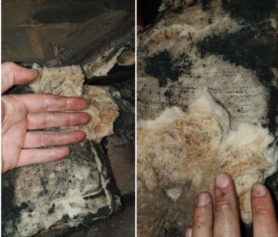
*Figure 6 - The insulation felt greasy after the fire*
