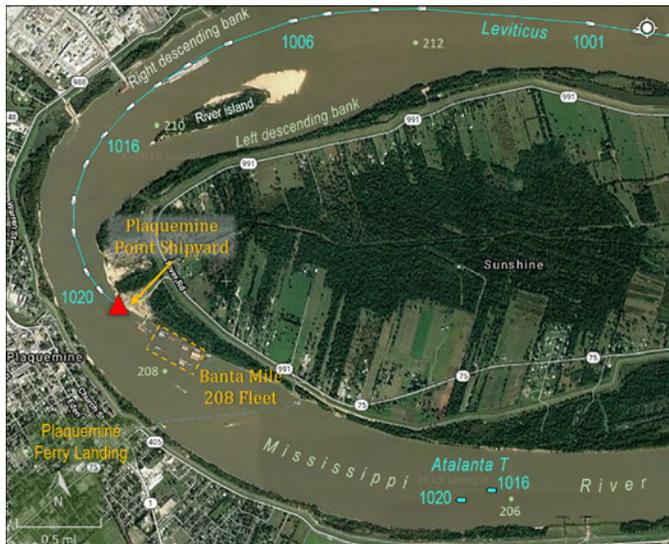
**Figure 96.** Trackline of *Leviticus* leading up to the contact with the barges moored at the Plaquemine Point Shipyard, based on the vessel's AIS data. According to the passing arrangement, Plaquemine Ferry Landing is where the tow would have met the *Atalanta T*.
