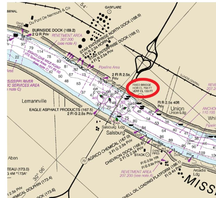
**Figure 93.** Excerpt of NOAA chart 11370 used by the crew. The vertical (133 feet) and horizontal clearances (750 feet) of the Sunshine Bridge are shown circled in red. SOURCE: NOAA; ANNOTATED BY NTSB.
