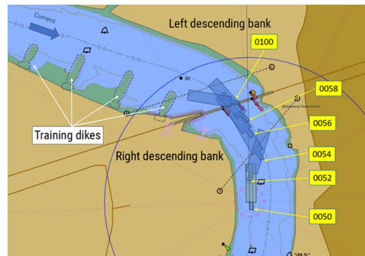
**Figure 116.** Select positions of the *Rivers Wilson* and barges on the Tombigbee River near mile 90 before the accident. Note the training dikes up river of the bridge on the right descending bank. BACKGROUND SOURCE: CORPS OF ENGINEERS; VESSEL DATA: GRAESTONE.
