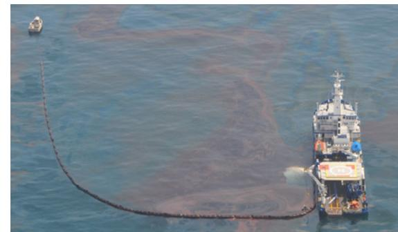
Figure 4. J-configuration deployment of oil spill boom by MSRC OSRV (right) and 32-foot workboat (left) during *Deepwater Horizon* oil spill response in May 2010.
