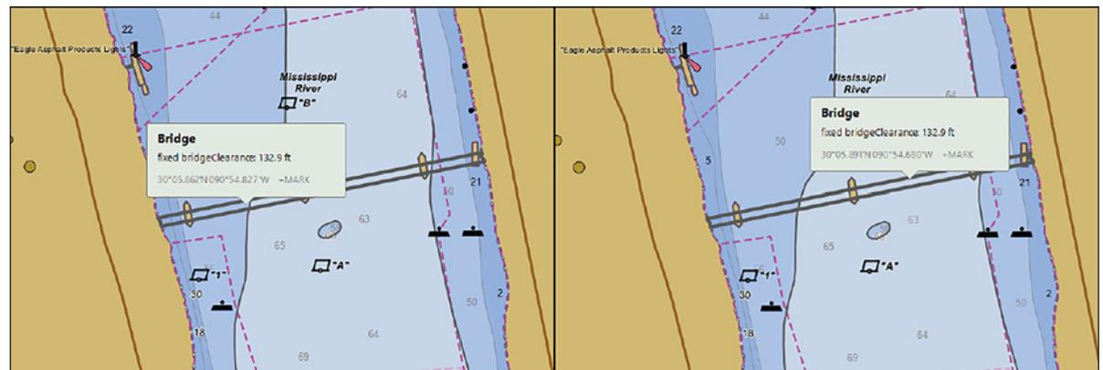
Figure 89. Vertical clearance of the Sunshine Bridge's west (left) and channel (right) spans, as indicated postaccident by the Rose Point display on board the *Kristin Alexis*, which showed the same clearance for each span (132.9 feet).
