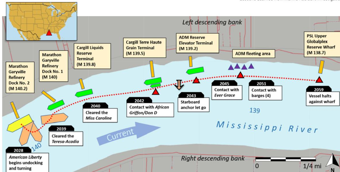
**Figure 48.** From where the *American Liberty* was moored, there were five wharfs on the left descending bank down river. All vessels were moored starboard-side-to, bow pointed upriver. Shown is the vessel's AIS track (red dots) getting underway, turning counterclockwise, moving bow first down river, and contacting vessels and wharfs along the left descending bank, as indicated by the red triangles. Not to scale. BACKGROUND SOURCE: GOOGLE MAPS.
