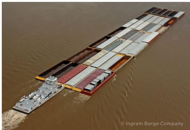
Figure 4. High horsepower towboat pushing 42 Jumbo barges.
