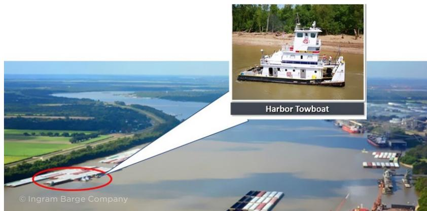
Figure A-1. Smaller “fleet boats” (circled in red) assembling barges for a tow.
