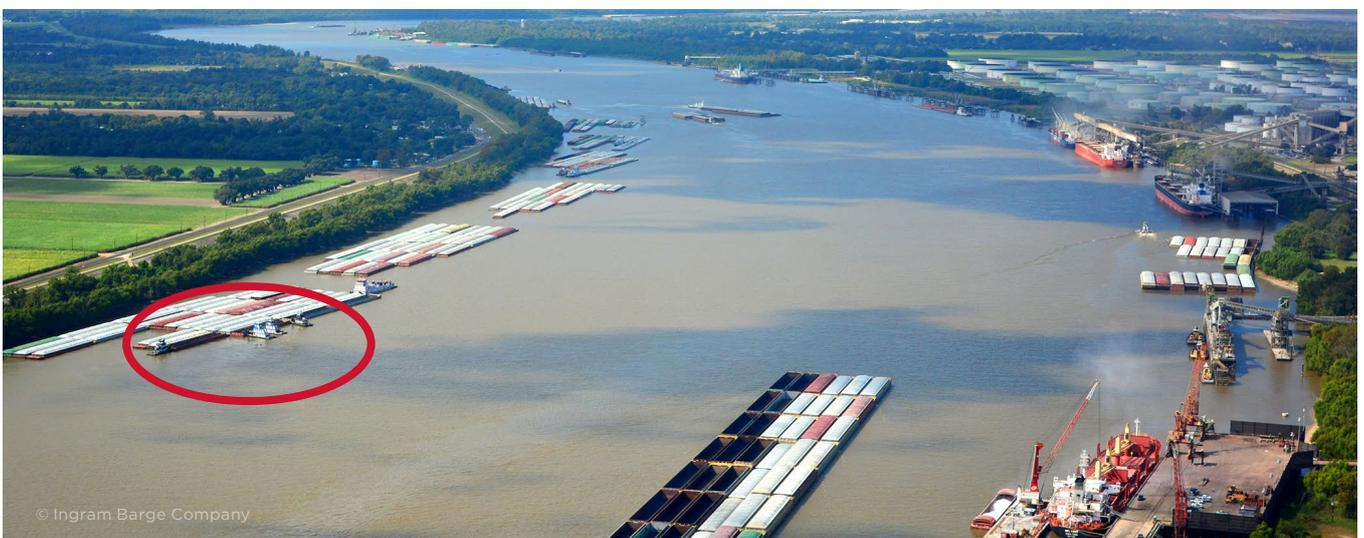
Figure 22. Smaller “fleet boats” (circled in red) assembling barges for a tow.
