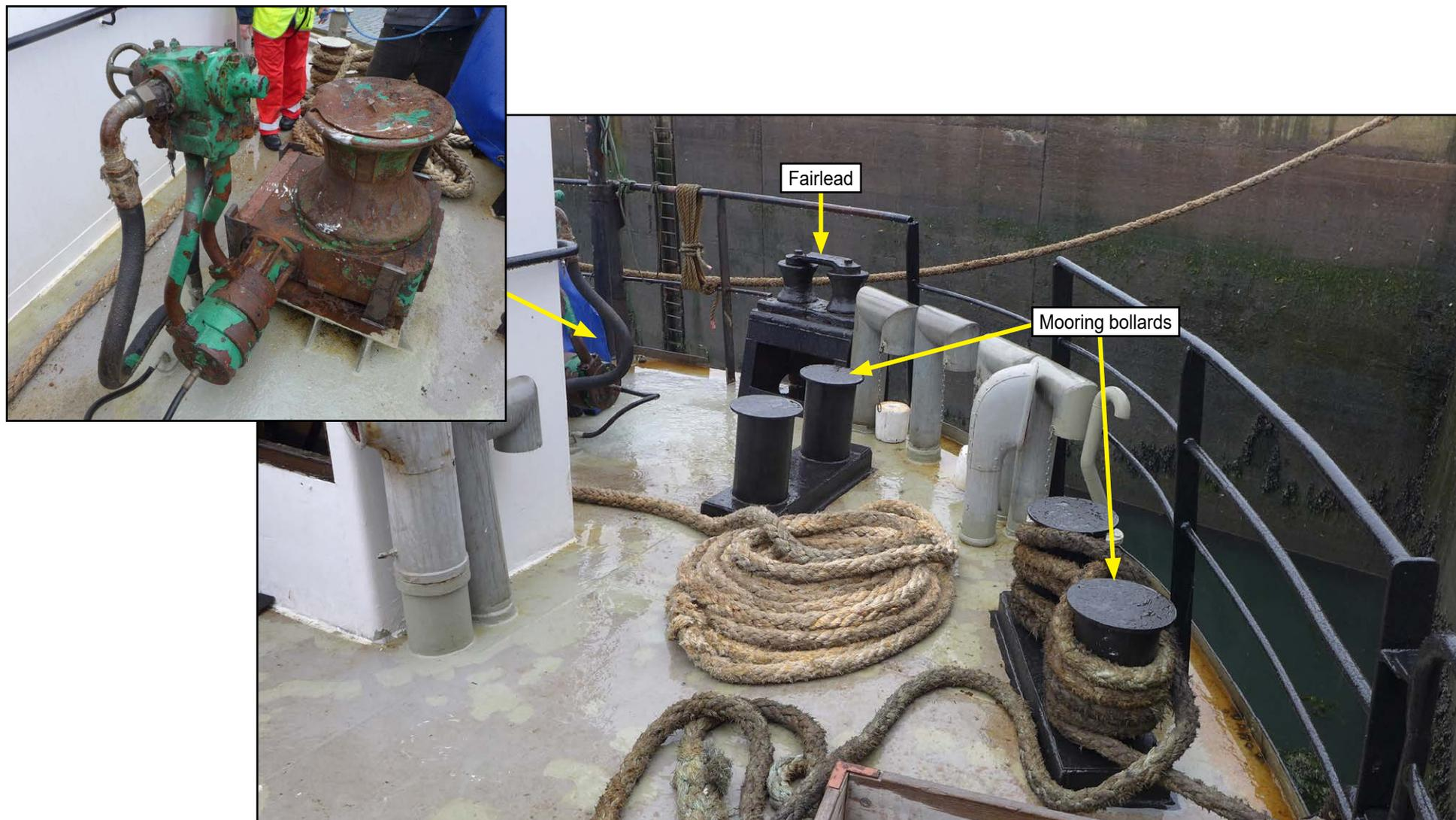
**Figure 7:** *Shearwater's* port side aft deck (looking aft) showing mooring equipment used for towing, with capstan inset
