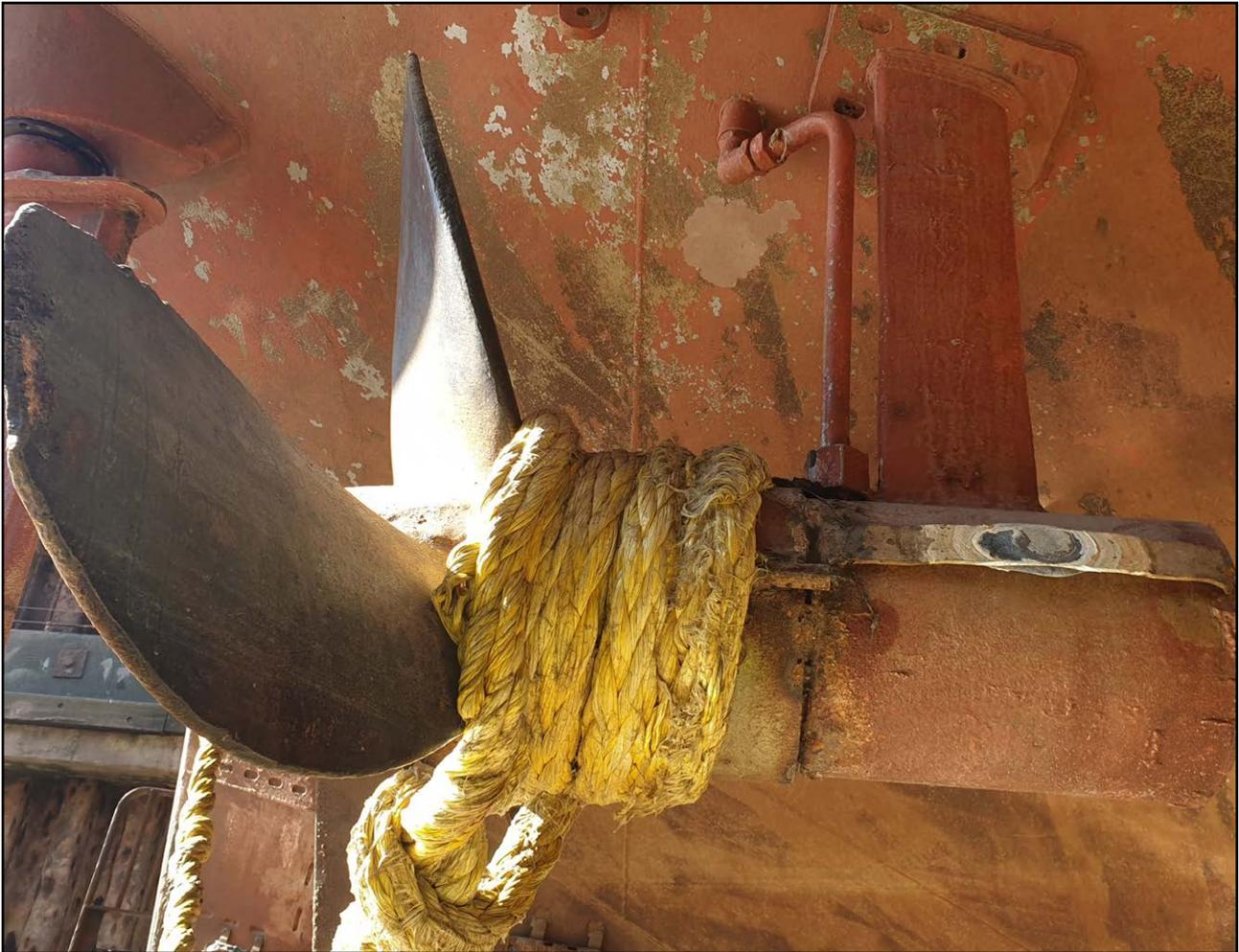
**Figure 6:** *Shearwater* in dry dock showing the towline around the starboard propeller
