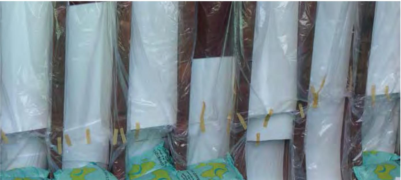
**Figure 3.8** | Styrofoam sheets are covered with plastic along the sideshell. Note that bags of rice can be loaded to touch the plastic sheeting so moisture from ship sweat cannot penetrate.
