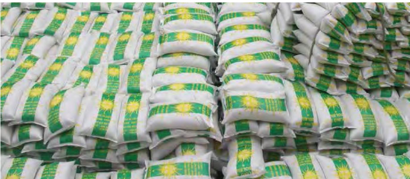
**Figure 4.8** | Note in the center foreground of the picture the bags laid across the ventilation channel running left to right interlocking the tiers. This is done so to stabilize the stacks of cargo preventing collapse and shifting of stacks.
