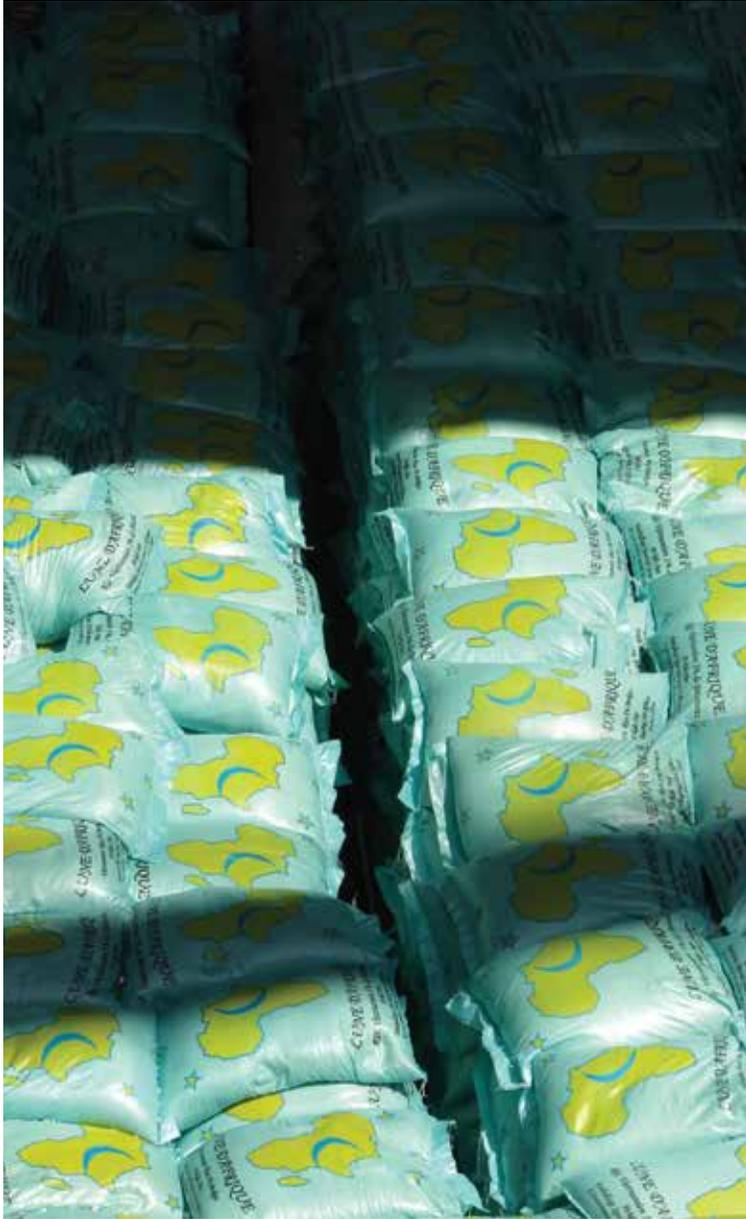
**Figure 4.2** | A ventilation channel in the cargo hold filled with bagged rice.
