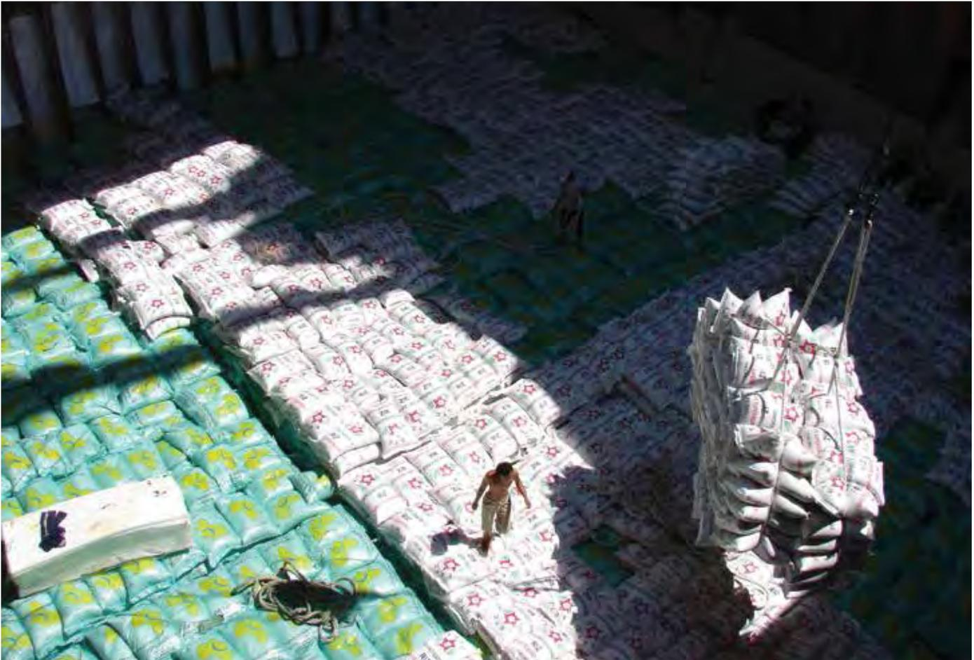
**Figure 4.1** | Stevedores loading and stacking bags with ventilation channels between stows. In the background, note the Styrofoam covered by plastic along the sideshells.
