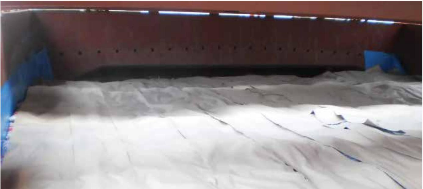
**Figure 3.15** | Cargo is loaded to the foot of the hatch coaming and covered with kraft paper. Also note the plastic sheeting protruding out of the sloping wing plates and taped to the hatch coamings.
