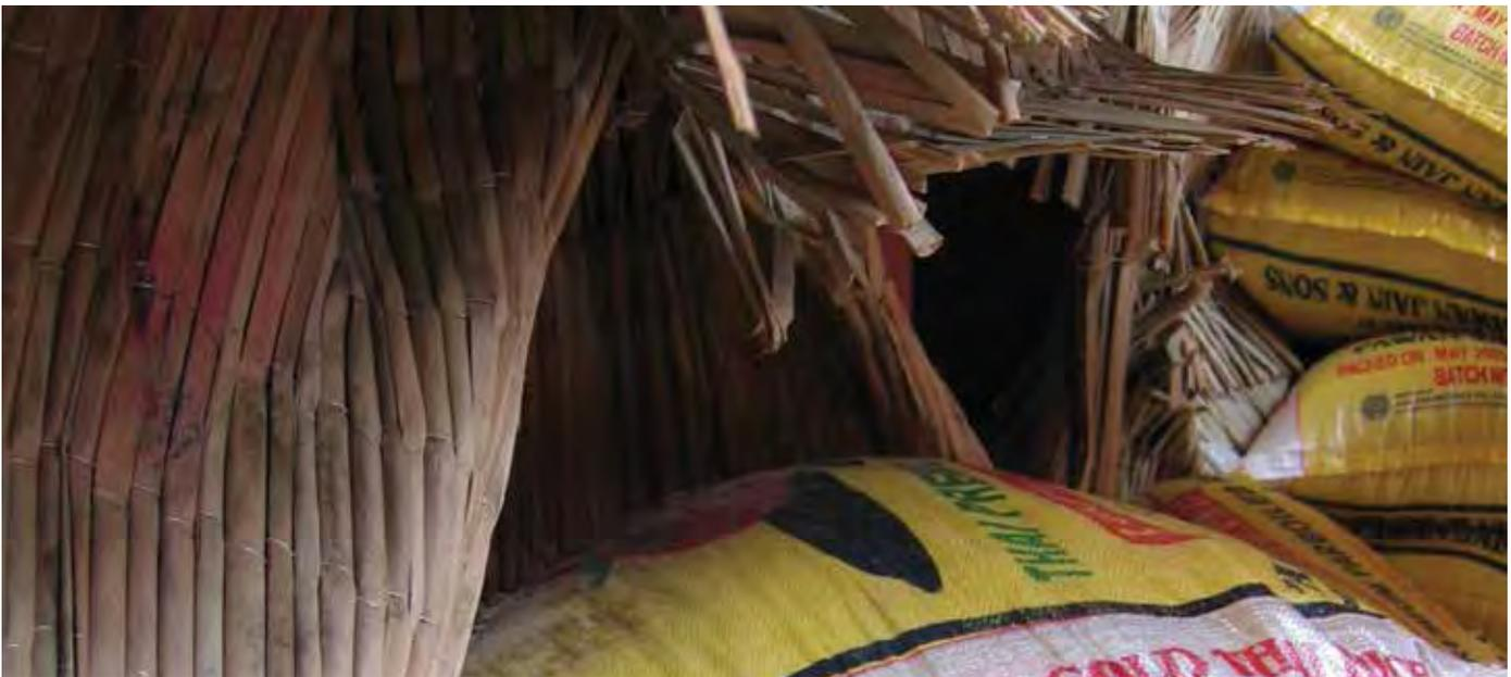
**Figure 3.4** | Bamboo mat dunnage placed along the ship sideshell has been stained by ship sweat. The bag adjacent to the dunnage has been stained as a result of the migration of water through the bamboo matting.
