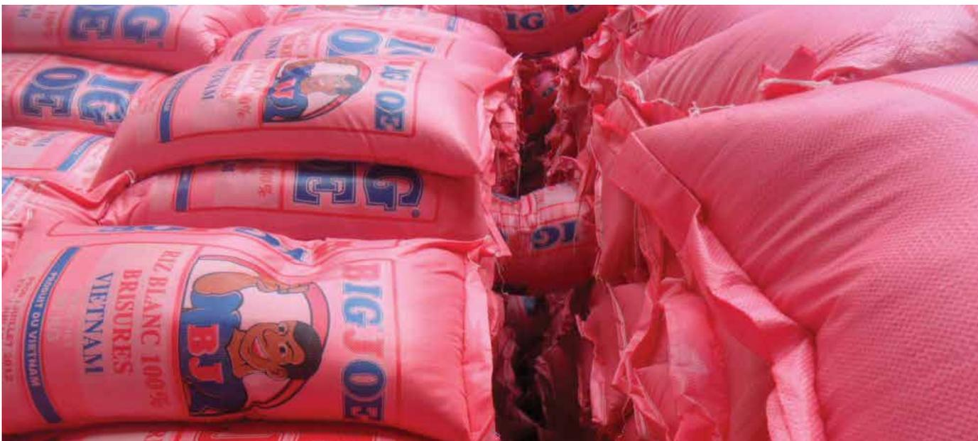
**Figure 4.7** | Ventilation channel between stacks of bagged rice. Note that every 5 or 6 tiers, that a rice bag is set across stacks interlocking the tiers. This is done so to stabilize the stacks of cargo preventing collapse and shifting of stacks.
