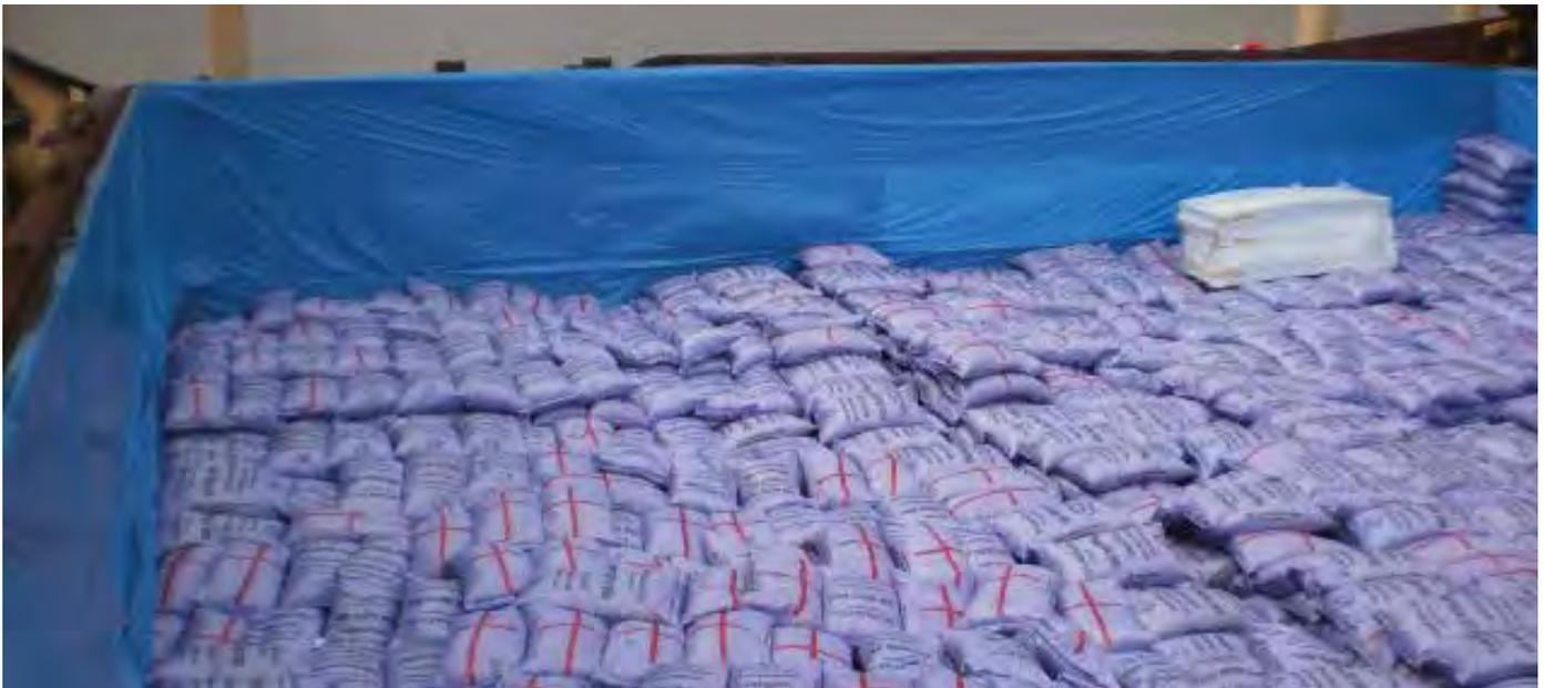
**Figure 3.14** | Cargo is stacked to the foot of the hatch coaming. Note the stack of Styrofoam sheets used for insertion between the hatch coaming and plastic sheeting.
