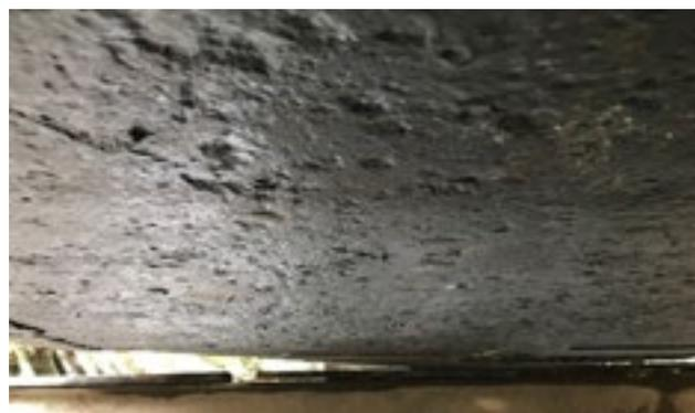
**Photograph 1. Galvanic pitting on the unpainted bottom of a Dutch Barge**
