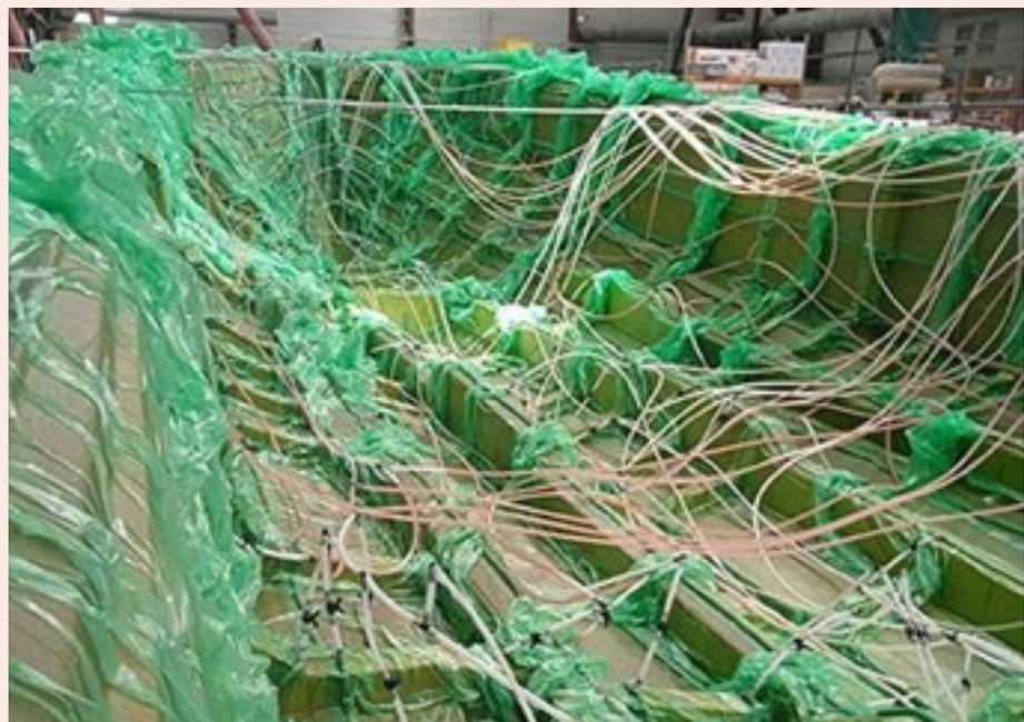
The hull of the new 26m Fly 86/2600 is the largest to date to be produced using Sicomin's GreenPoxy bio-epoxy system. "Our InfuGreen 810 resin really does offer the optimum solution for infusion in a large structure such as the Fly 86/2600," said Philippe Gruaud, head of technical sales for western France, Sicomin.
