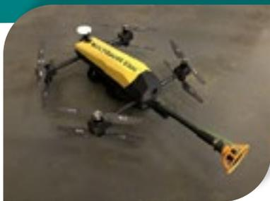
*The Drone Thickness Gauge*
