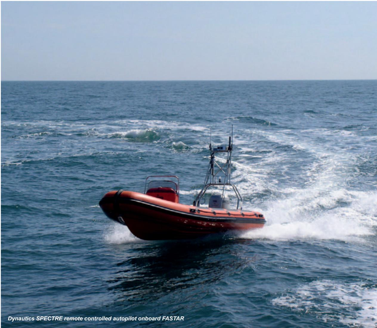
*Dynautics SPECTRE remote controlled autopilot onboard FASTAR*
