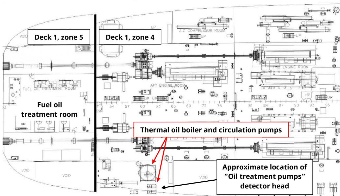
**General arrangement plan with “oil treatment pumps” and fuel treatment room identified**
