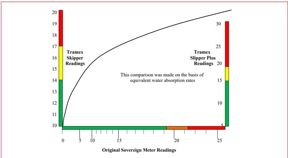
Figure 1 - Approximate Comparisons of Moisture Meter Readings
