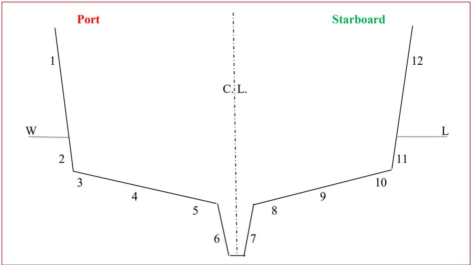
Figure 3 - Sketch of Boat's Midship Section showing Position of Readings
