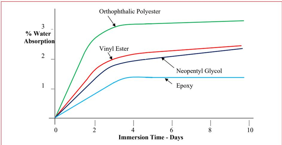
Figure 2 - Typical Water Absorption Curves
