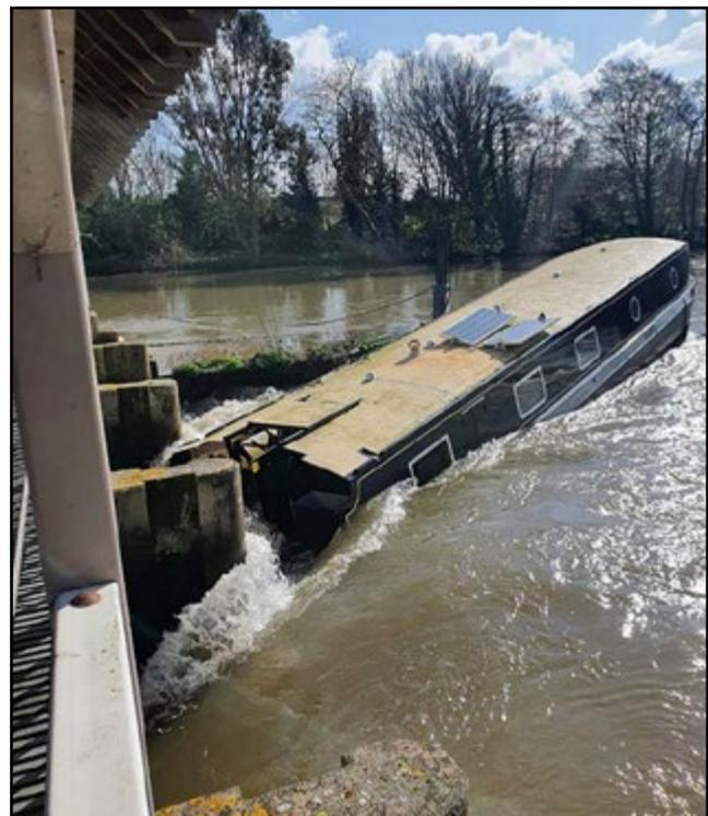
Figure 1: Narrowboat partially sunk on weir
