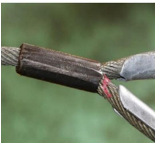
Figure 3: Fitting is deformed with "ridges" of extra material present from over-crimping.
