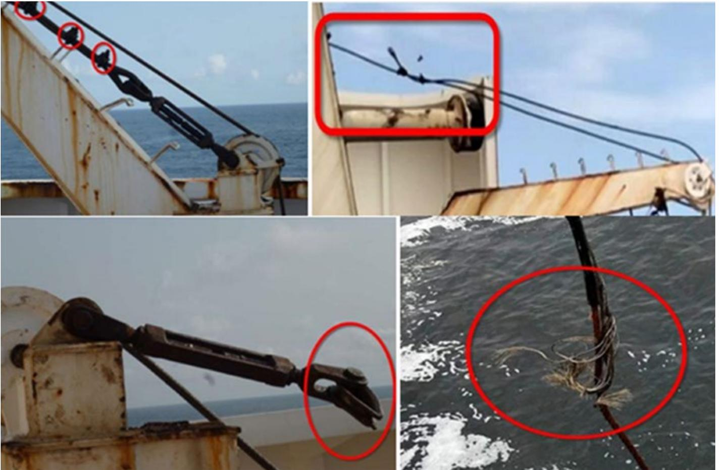
During a five-yearly 110% load test of a lifeboat, taking place under third party supervision, the forward fall wire failed, resulting in the lifeboat falling and flipping upside down landing in the water below. There were no personnel onboard during testing and no injuries were reported. The lifeboat was recovered to shore.
