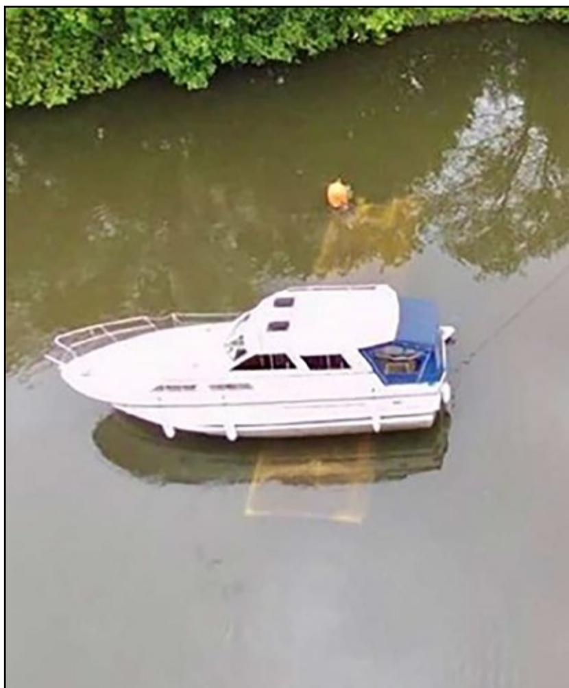
Figure 2: Motor cruiser grounded on submerged wreck
