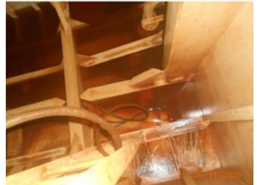
During inspection of a fresh water tank, it was discovered that there was significant sludge accumulation in the tank. Based on the condition of the tank, it was seen as more than likely that other tanks would be similarly affected and that the cause was due to a common source of water. Sludge build-up in fresh water tanks, hoses and pipes can lead to the prevalence of bacteria that may pose a health hazard.
