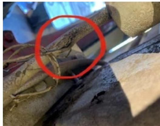
During a washdown of a vessel's cargo hold a crew member noticed arcing from around two electrical cables near the cargo hold light. Upon closer investigation he noticed a piece of tie wire connected to the cables was glowing red. The crew member immediately stopped hosing down and turned the water supply off and notified the ship's electrician.
