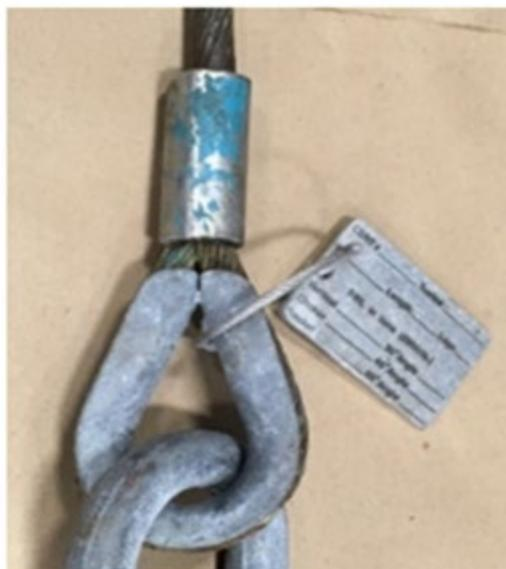
Figure 1: Fitting has a uniform appearance.
