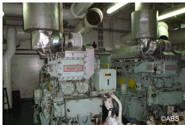
Auxiliary engine exhaust insulation renewed
