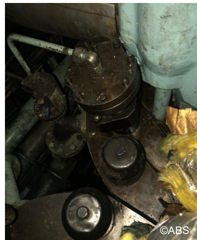
Faulty Starting Valve replaced by spare
