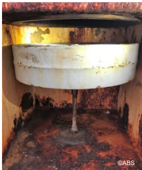
Air pipe float found defective
