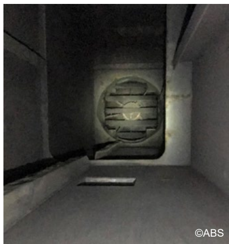
Engine room fire damper found defective
