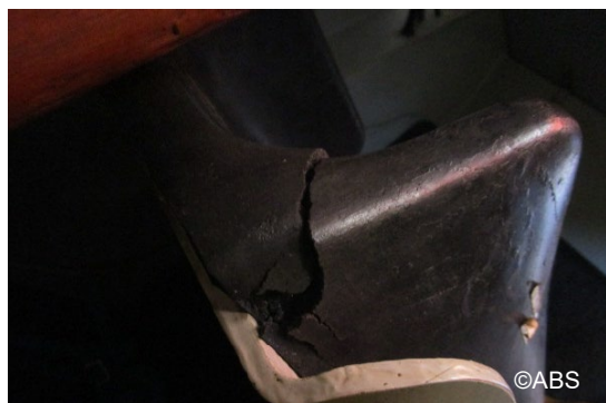
Lifeboat Free Fall seat partly broken
