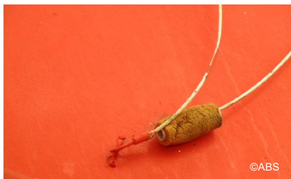
Lifeboat grab line floats damaged – before
