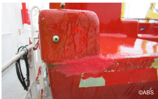
Rescue boat hull minor crack (stern)
