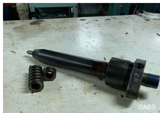
Main engine broken spring for fuel valve found
