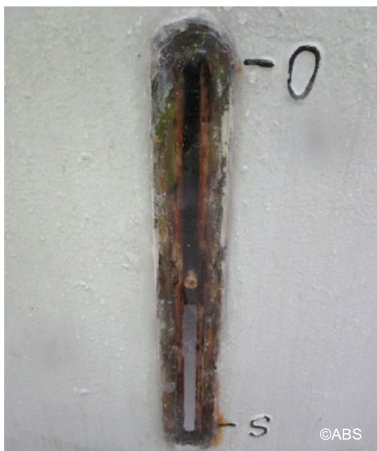
Ventilation funnel from EDG indicator of position not covered
