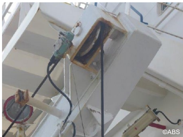
Lifeboat limit switch malfunction
