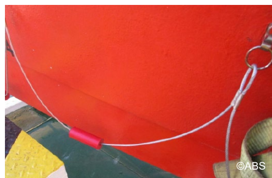
Lifeboat grab line floats damaged – after
