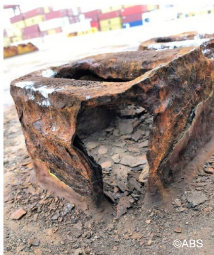
Wasted container socket - before
