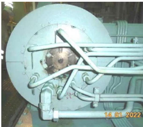
**Figure 7.** The main engine's starting air distributor containing the no. 6 starting air actuator valve. (Source: Thome Ship Management)
