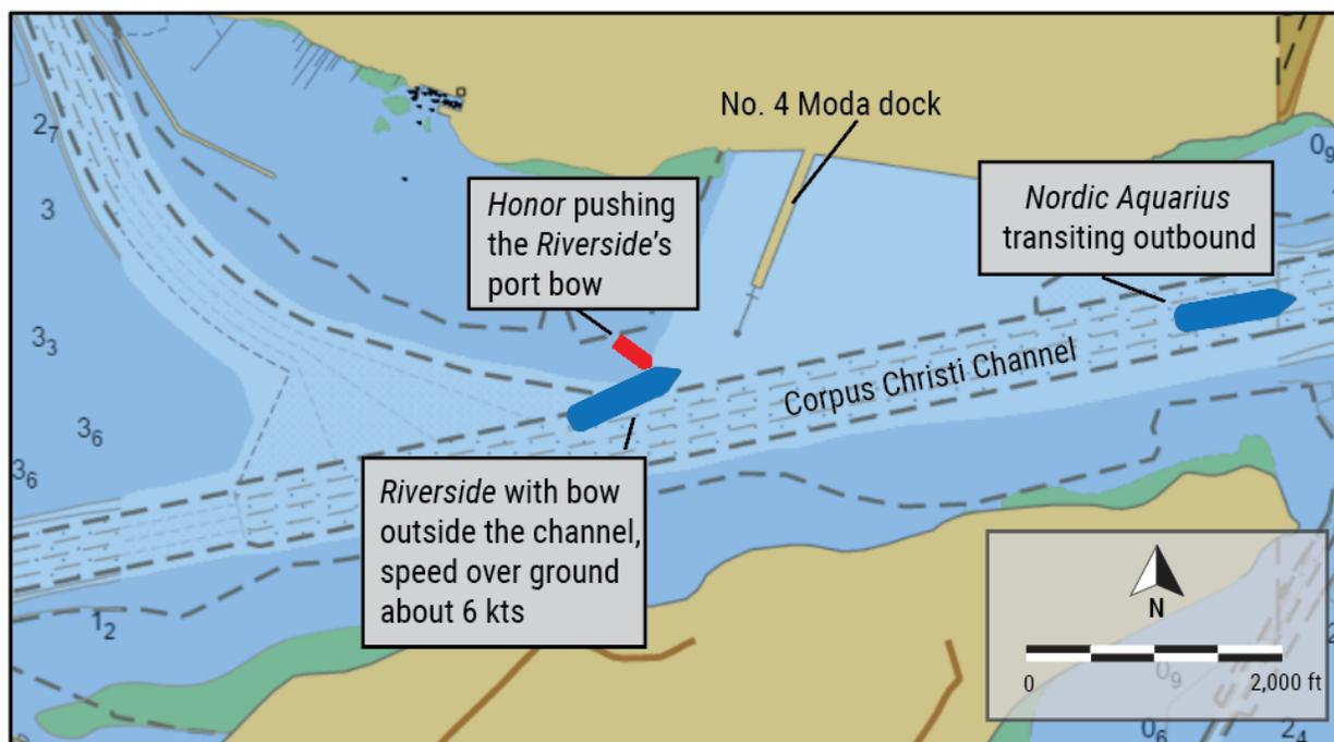
**Figure 4.** Approximation of *Riverside* at 1300, just before the contact with the no. 4 Moda dock dolphin and catwalk, with the tug *Honor* pushing its port bow; the *Nordic Aquarius* has departed the no. 4 Moda dock and is transiting outbound. (Background source: NOAA)
