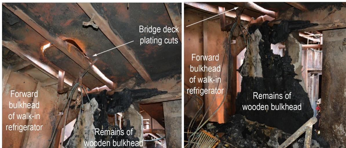
**Figure 8.** Forward end of *Aleutian Falcon* walk-in refrigerator after the fire. (Background source: ATF)
