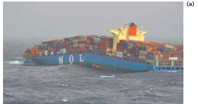
Image 9 (a) and (b): MOL Comfort (8,100 TEU, 2013, total ship loss in the Arabian Sea), broken in two following primary hull girder failure.
