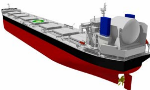
Figure 123: Tsuneishi Shipbuilding’s LNG fuelled bulk carrier design – Kamsarmax GF.
