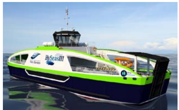
Figure 129: HySeas III – the third development stage of EU funded project to deliver a ferry powered by hydrogen fuel cells.
