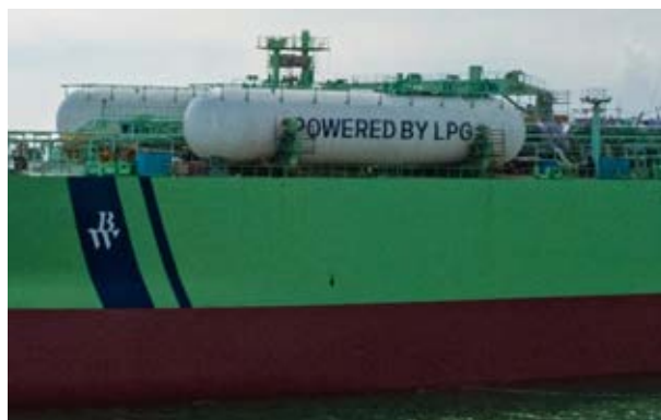
Image 22: BW MV Gemini, LPG fuel tanks.
