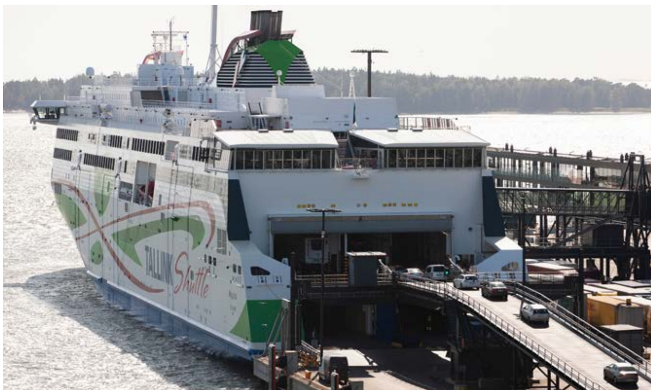
Image 1: Ro-ro passenger ship - main deck openings and superstructure.
