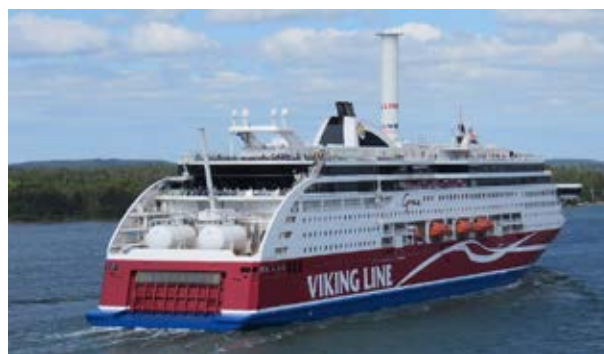
Image 13: MV Viking Grace – LNG fuelled RoPax represents still one of the world first LNG fuelled flagships, operating since 2013.
