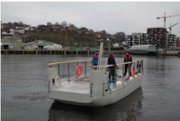
Image 12: The full-scale autonomous ferry prototype milliAmpere II.
