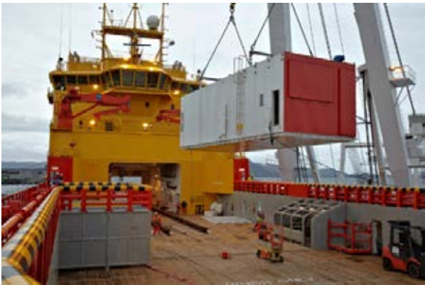
Figure 138: Viking Lady embarking fuel cell power module in the context of the FellowSHIP project.
