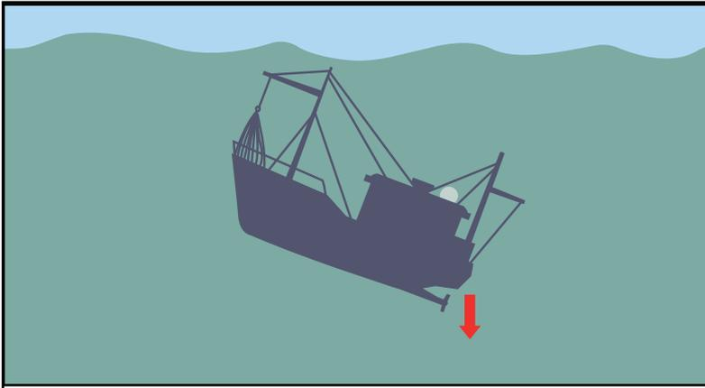
As the Hydrostatic Release Unit sinks below the depth of operation, it activates and severs the rope securing the liferaft canister to the cradle
