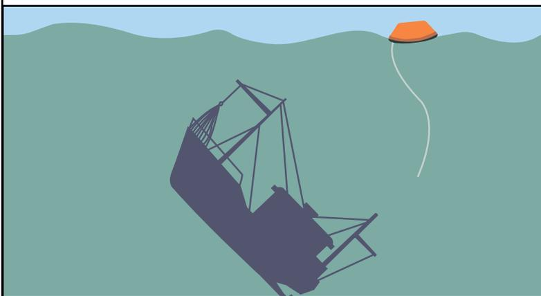
The buoyancy of the the inflated liferaft overcomes the breaking force of the weak link and the liferaft floats to the surface
