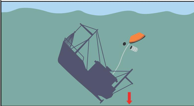
When the painter line has been pulled out to its entire length, the actuator wire activates the inflation system
