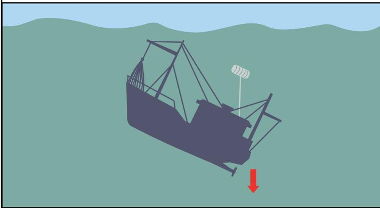
The liferaft canister releases from the cradle and inherent buoyancy in the uninflated liferaft pulls out the painter line
