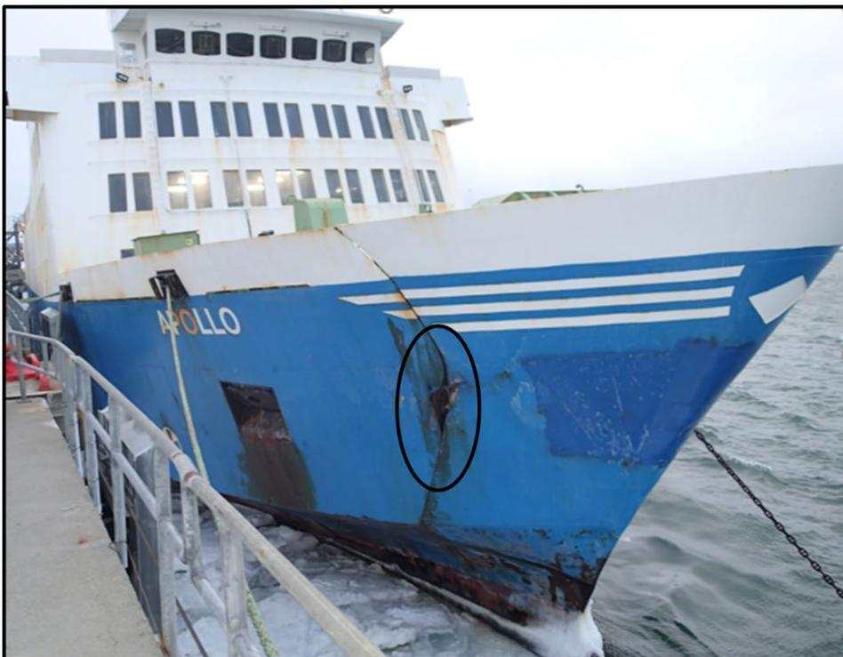
Figure 5. Damage to the Apollo (circled) (Source: TSB)
