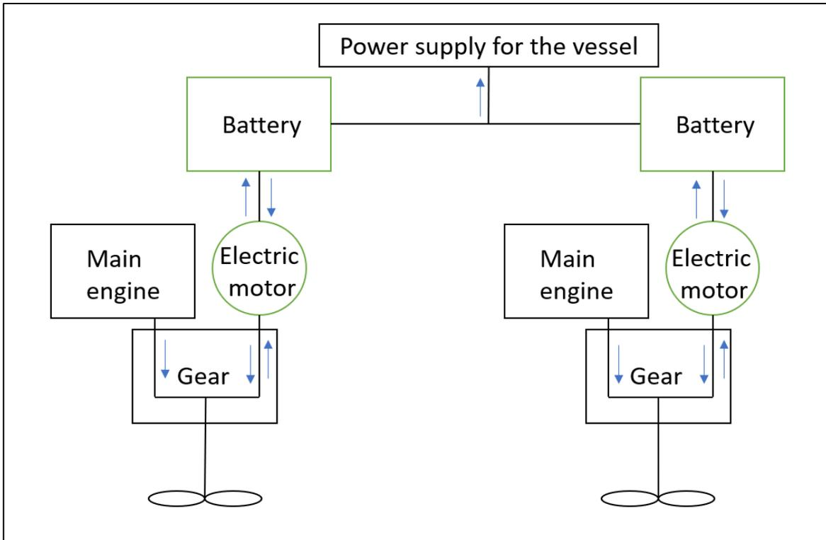
Figure 12: Hybrid propulsion system. Illustration: NSIA
