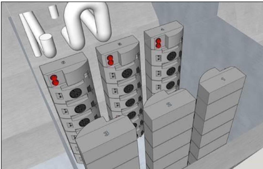
Figure 3: Six stacks of battery modules in one of the battery rooms. Illustration: The battery contractor
