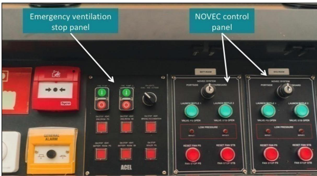
Figure 25: Novec panel on the bridge. The key on the right controls the fire suppression system in the engine rooms, while the key on the left controls the system in the battery rooms. Photo: Shipping company
