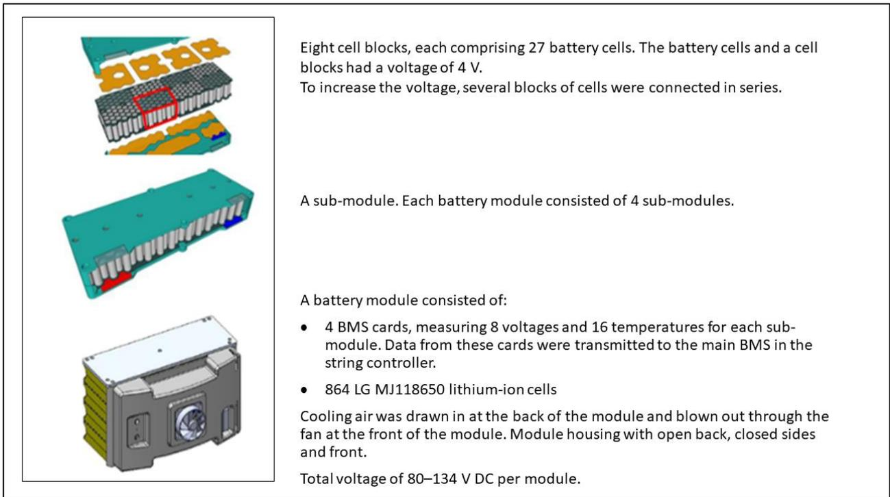
Figure 17: Battery module design. Illustration: The battery contractor
