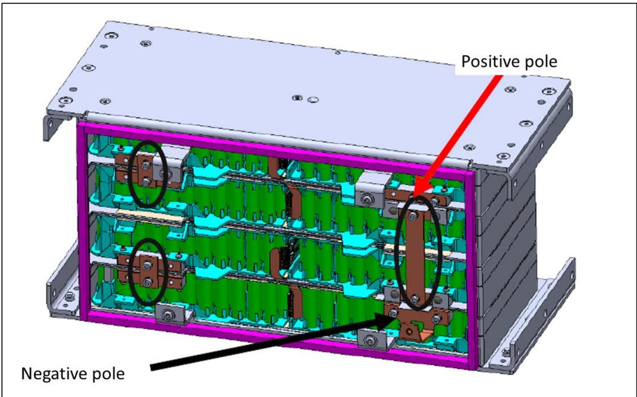
Figure 16: Connection of the sub-modules with indication of the connection points, the module's positive and negative poles. The copper strips are shown as vertical rectangles and marked with a black circle. The negative and positive poles are marked with arrows. Illustration: FFI/NSIA/The battery contractor
