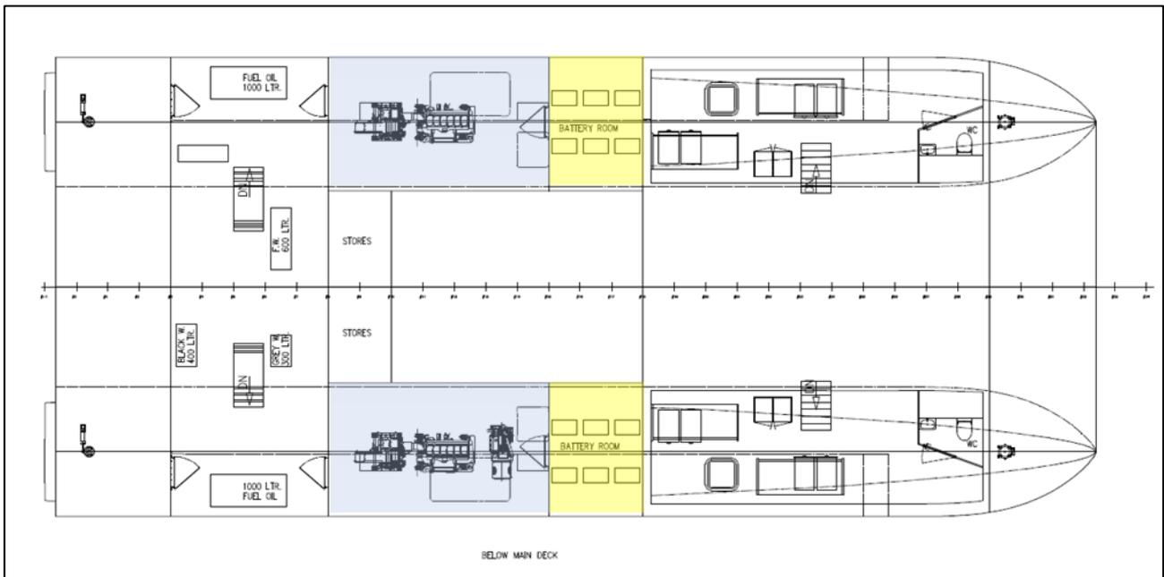
Figure 13: GA drawing showing the location of the engine rooms (blue) and battery rooms (yellow) below the main deck. Technical drawing: The shipyard
