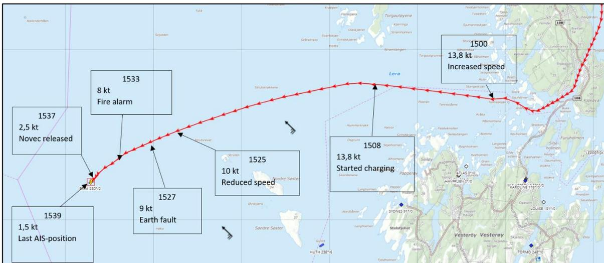
Figure 2: AIS track of the vessel's voyage. The times are those observed by the crew, based on interviews and the EMS log, but differ from the times registered by the battery management system (BMS). Map: The Norwegian Coastal Administration/NSIA
