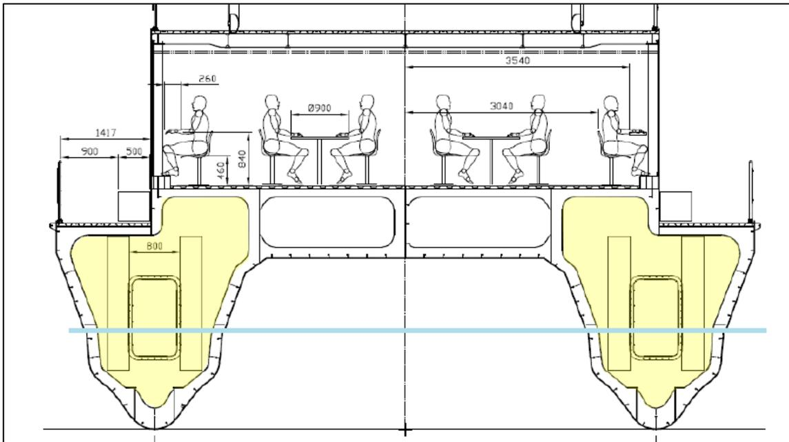
Figure 14: The battery rooms (yellow) seen in relation to the waterline (marked in blue). Technical drawing: The shipyard
