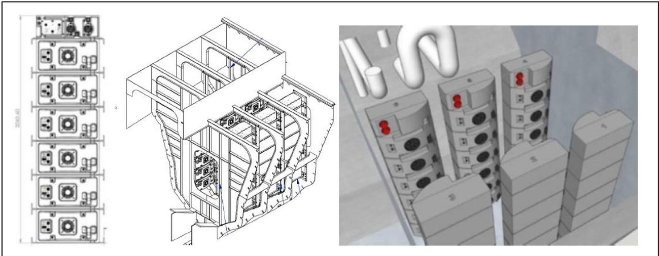
Figure 15: The drawing on the left shows a stack of six battery modules with a stack controller at the top. The middle and right-hand drawings show six battery stacks in one battery room. Illustration: The shipyard
