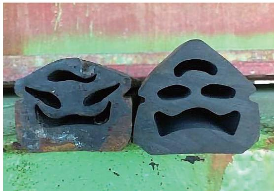
Photograph 9 Overcompressed CAT seal
