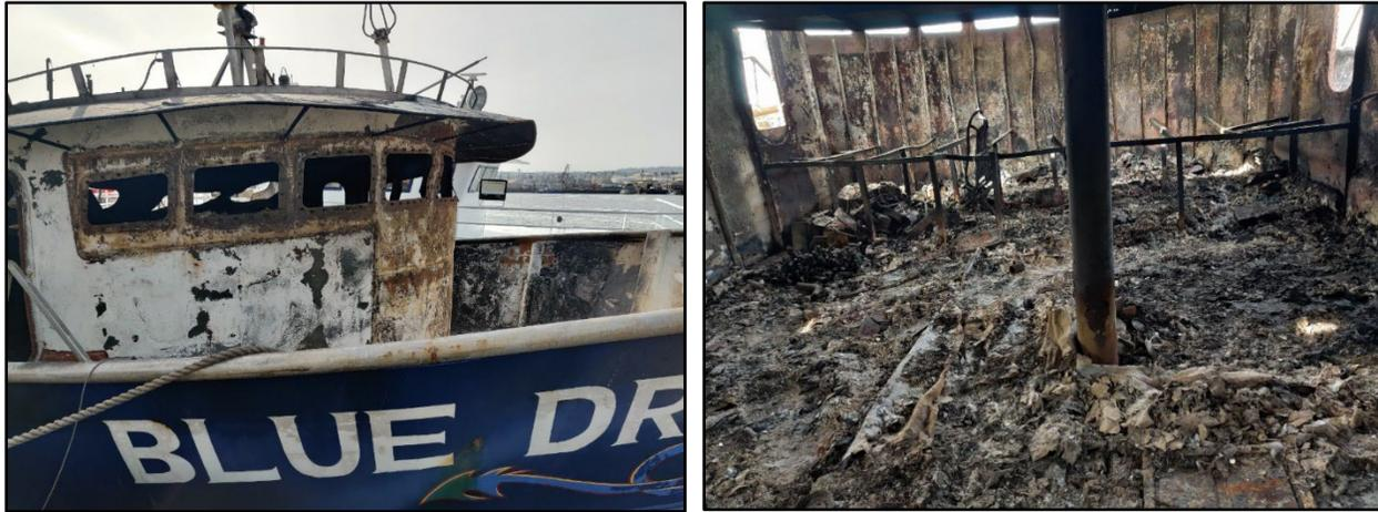
**Figure 6.** *Blue Dragon* wheelhouse exterior (left) and interior looking forward (right), after the fire. The framing of the false deck in right image indicates the location of what was the wheelhouse deck. (Source: Coast Guard)
