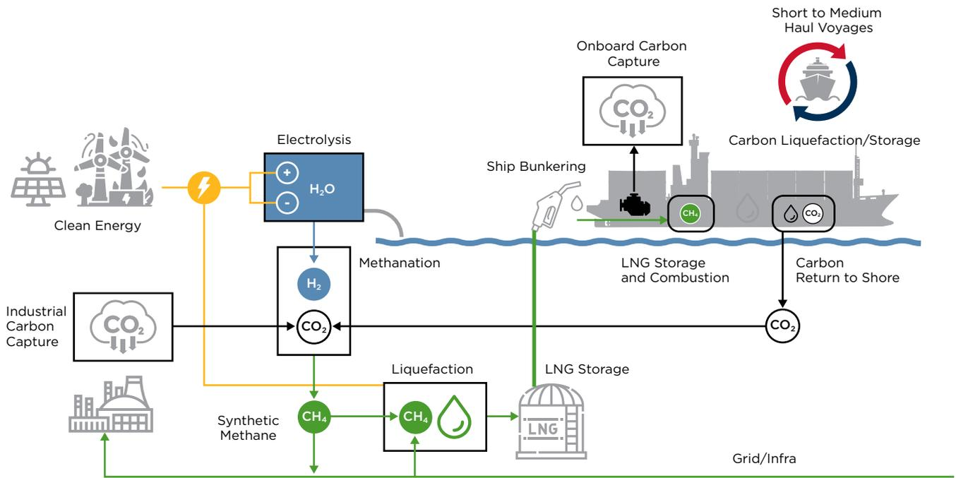
Figure 5: Case Study for CO<sub>2</sub> Carbon Capture on an LNG-fueled RoPax Ferry
