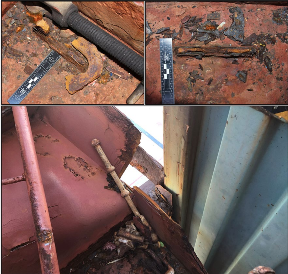
Figure 8: Thinned, heavily wasted and failed lashing eyes (top) and wasted and failed container support structure (bottom) from bay 62
