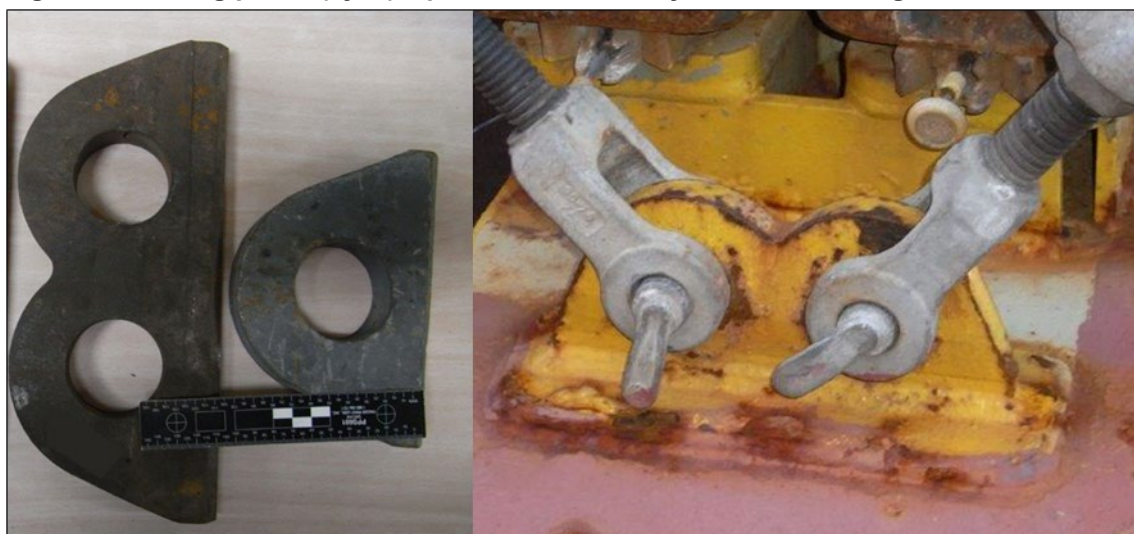
Figure 4: Lashing plates (eyes), spare and as recently fitted to APL England
