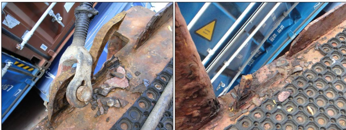
Figure 7: Typical, thinned, heavily wasted and failed double (left) and single (right) lashing eyes from bay 30
