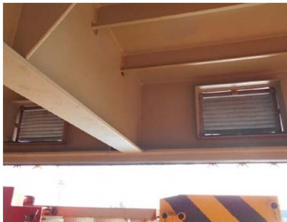
Figure 2: Internal view of hinged-door ventilator on cargo hold hatch cover side (photo courtesy of Optimum Marine Management Ltd.)
