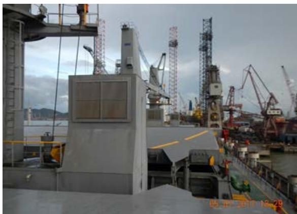
Figure 7: External view of mechanical ventilation casing with louvre on the main deck (photo courtesy of Ionic Shipping (Mgt) Inc.)
