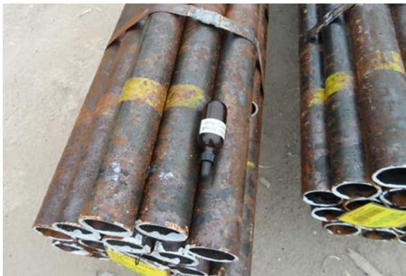
Figure 13: Surface corrosion or rust due to cargo sweat (photo courtesy of The Standard Club)
