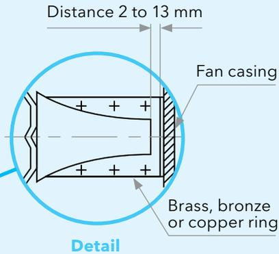
Figure 24: Example of non-sparking design
