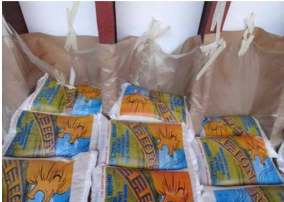
Figure 28: Layers of Styrofoam, kraft paper and plastic sheeting (photo courtesy of OLDENDORFF CARRIERS GmbH & Co. KG.)
