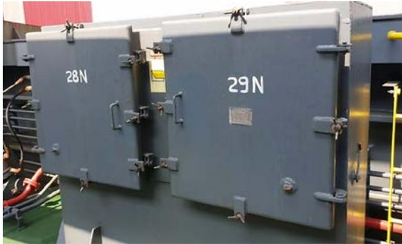
Figure 3: Hinged-door natural ventilator in casing on main deck (photo courtesy of OLDENDORFF CARRIERS GmbH & Co. KG.)
