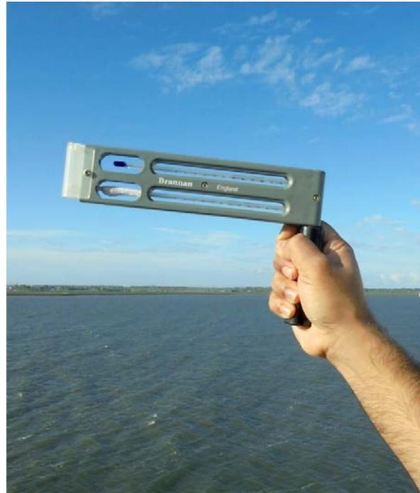
Figure 20: Whirling psychrometer in use (photo courtesy of Fleet Management Limited)
