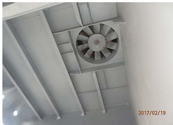
Figure 8: View of cargo hold mechanical ventilation impeller from inside the cargo hold - cross-deck (photo courtesy of Ionic Shipping (Mgt) Inc.)
