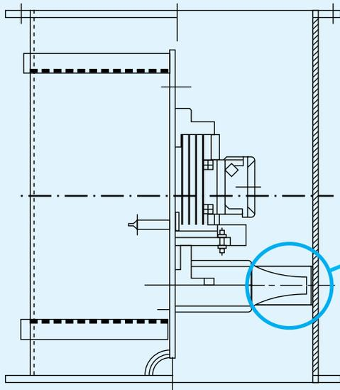
Figure 23: Example of non-sparking design
