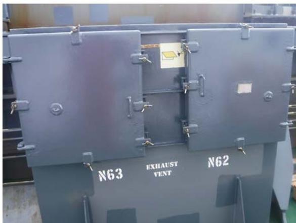
Figure 6: Hinged-door mechanical ventilation - exhaust vent (photo courtesy of OLDENDORFF CARRIERS GmbH & Co. KG.)
