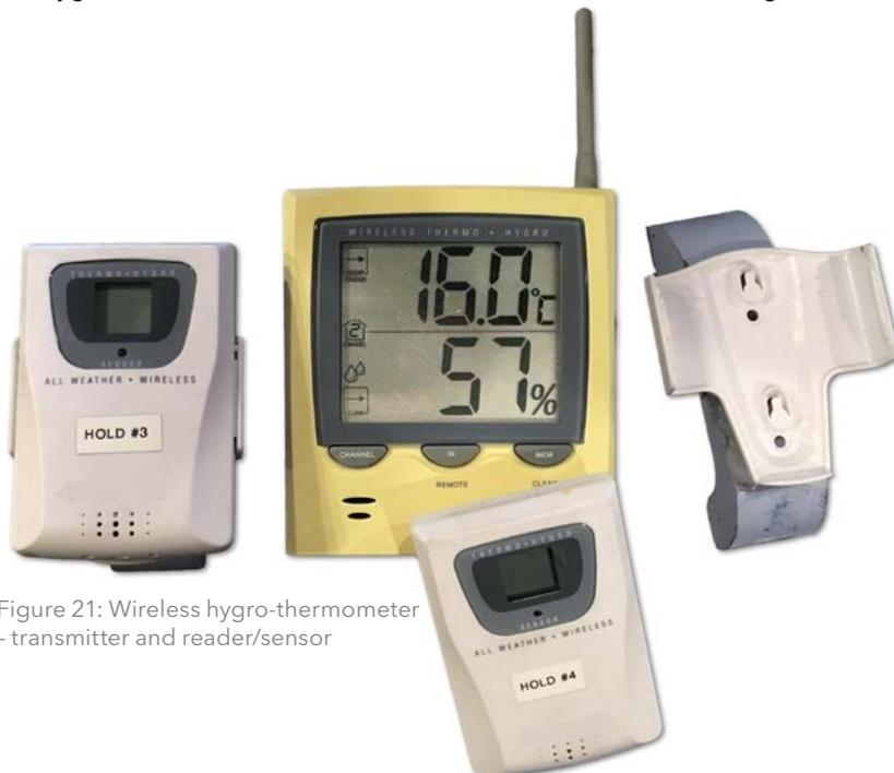
Figure 21: Wireless hygro-thermometer - transmitter and reader/sensor
