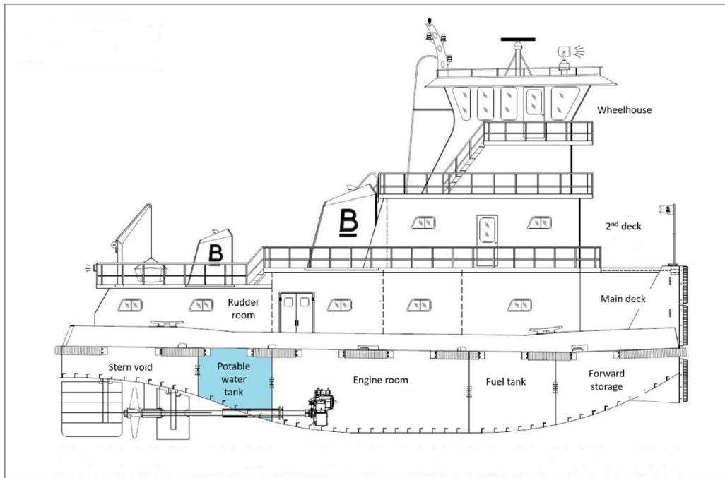
**Simple profile of the *Alton St. Amant* (not to scale), with the potable water tank highlighted. (Source: Blessey Marine Services; annotated by NTSB)**
