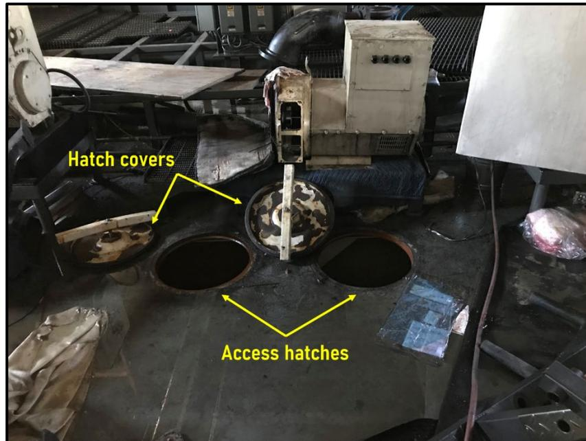
Open access hatches and their covers for the two potable water tanks in the rudder room. (Source: Coast Guard)
