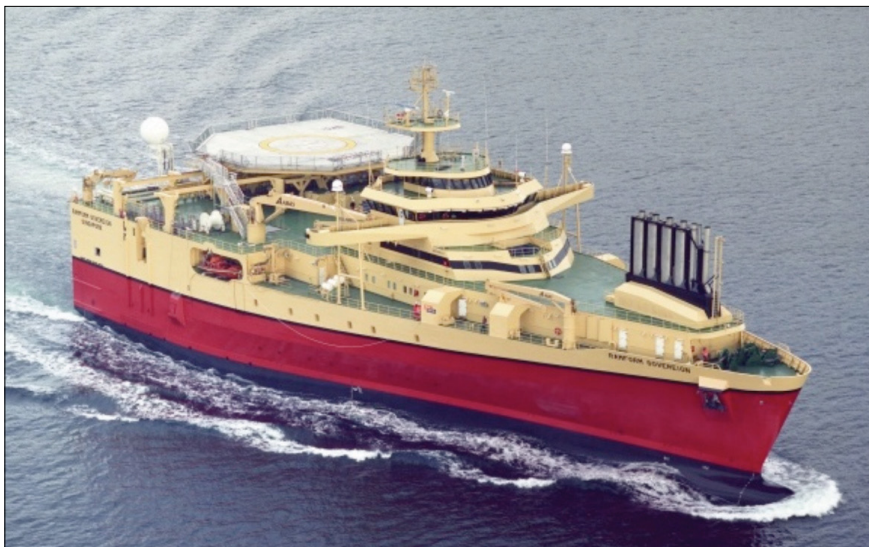
New generation Ramform Seismic vessel (note the stern breadth)
