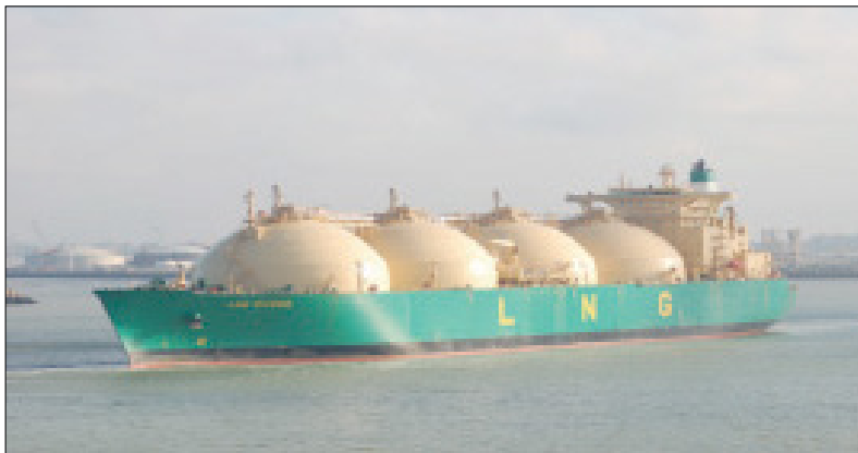
LNG carrier of 135,000m 3 (note the spherical tanks)
