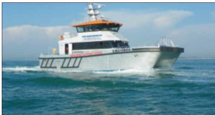
Aluminium wind farm support vessel (note the bow transfer arrangement)
