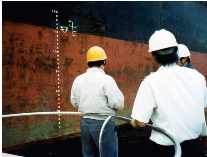
Reading draught marks using a boat
