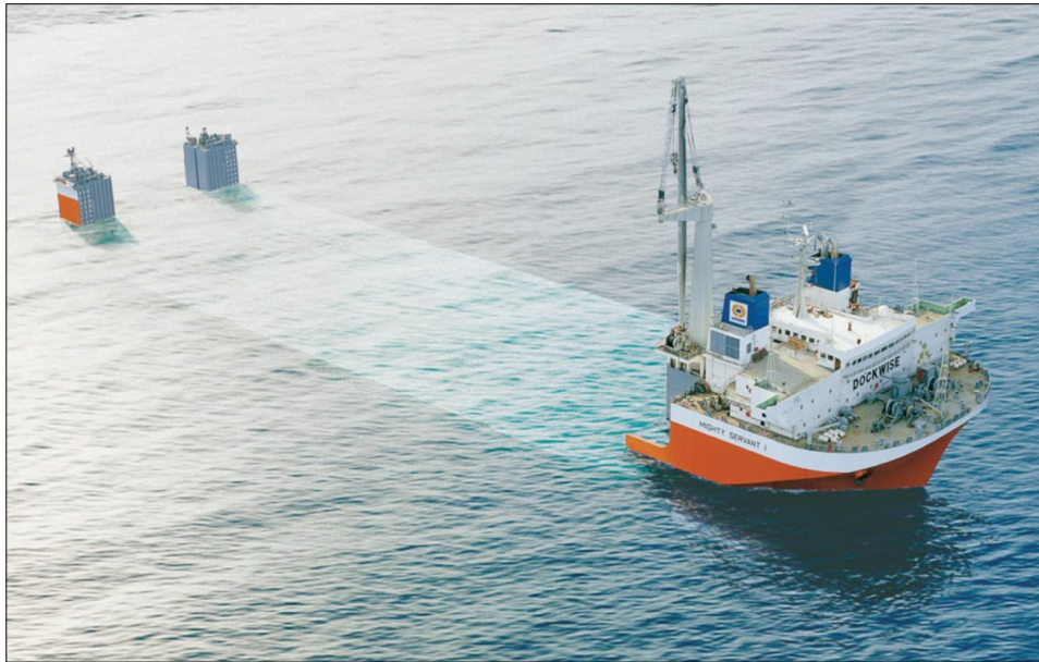
Mighty Servant I in submerged mode awaiting cargo float over
