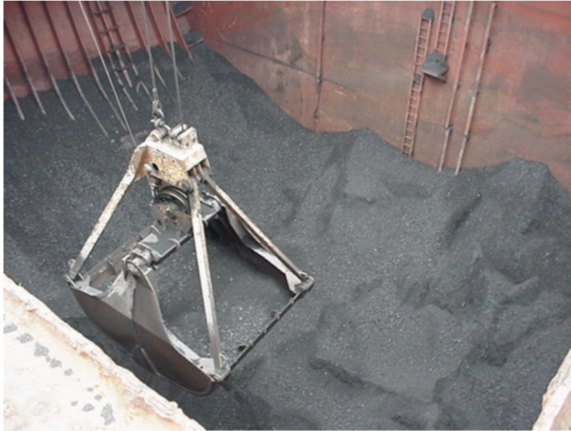
Discharging coal using mechanical grabs
