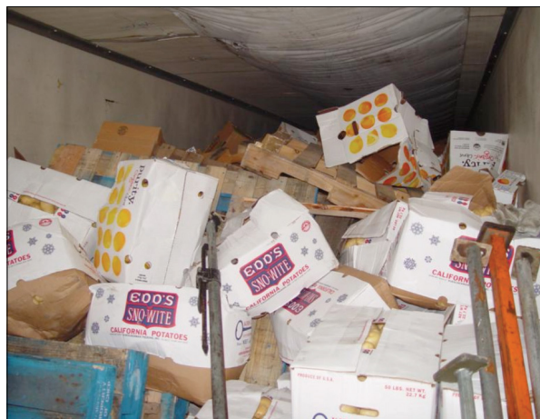
Serious damage to cartons of potatoes due to initial poor stowage
