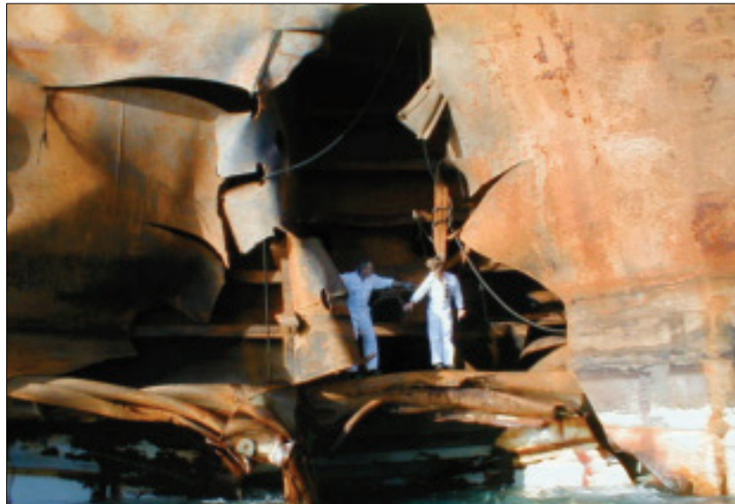
Serious structural hull damage following a terrorist attack
