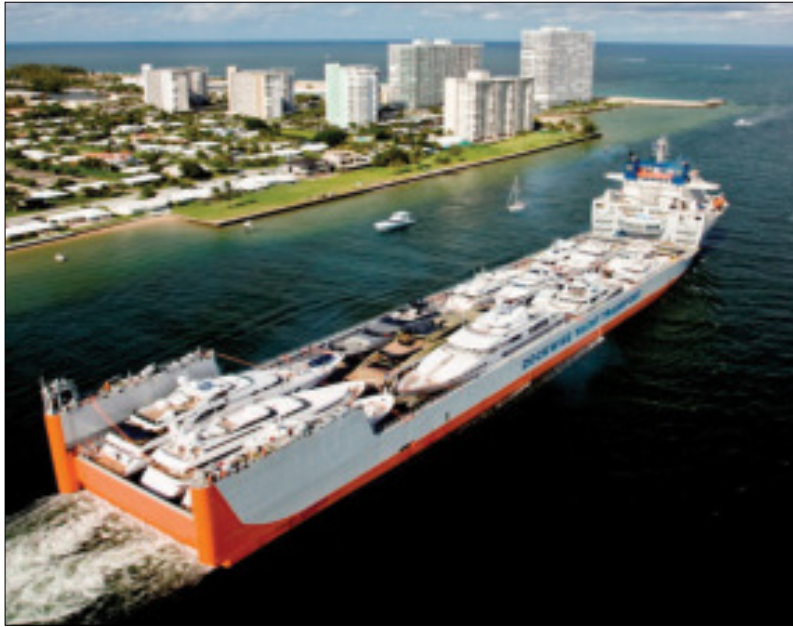
Yacht Express a special semi-submersible yacht carrier
