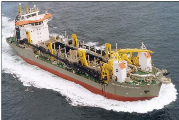
Coastal suction dredger (note the suction pipes)
