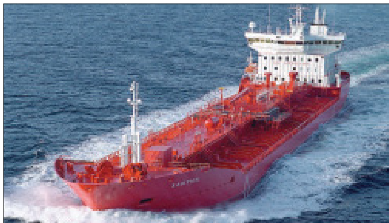
Typical chemical tanker of 17,000 dwt
