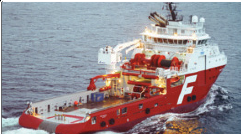
AHTS Far Saracen (note stern roller and winch system)
