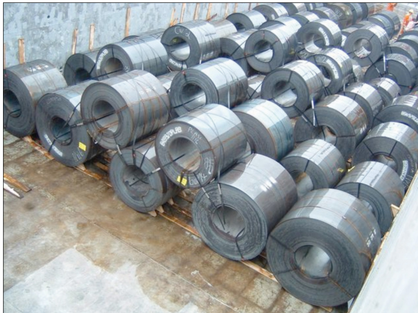
A well stowed cargo of steel coils showing the locking coils, proper dunnage and chocks all secured using hydraulic banding
