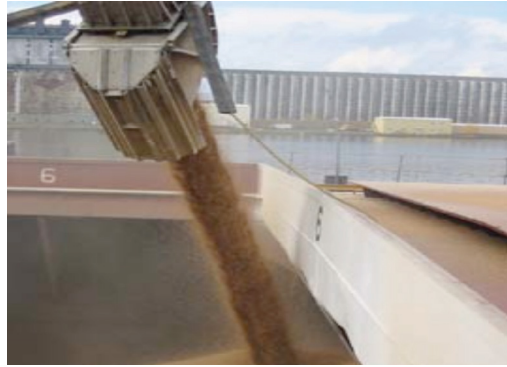
Loading grain from a silo using a mechanical loader
