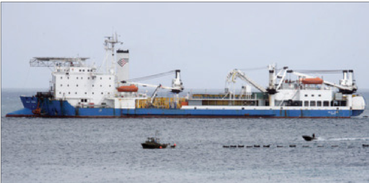
Modern cable layer (note the midships carousel)
