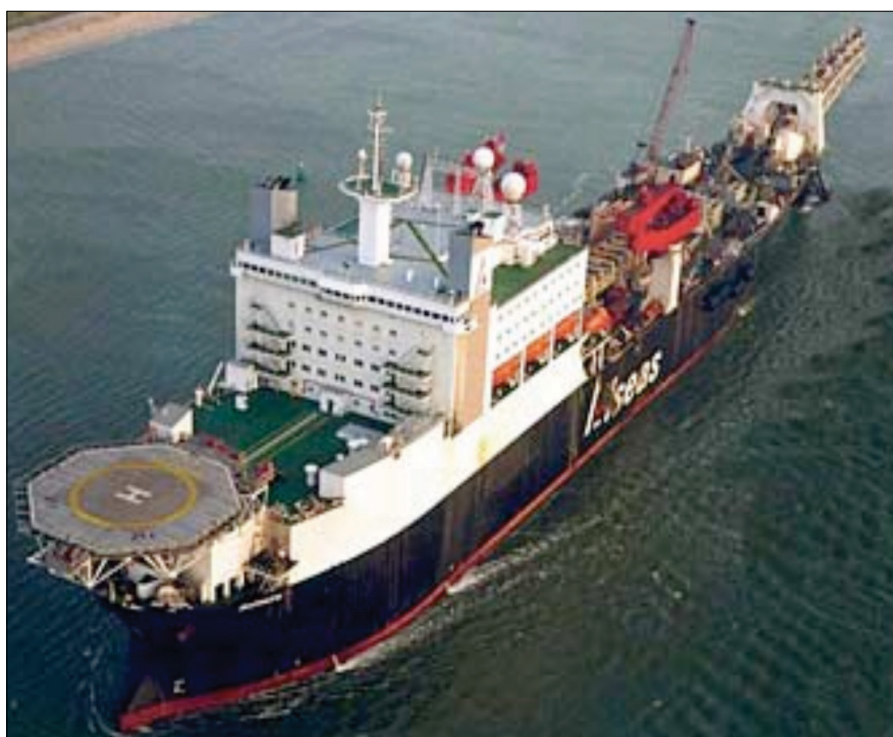
New generation mono hull pipe lay vessel (note the stinger aft)
