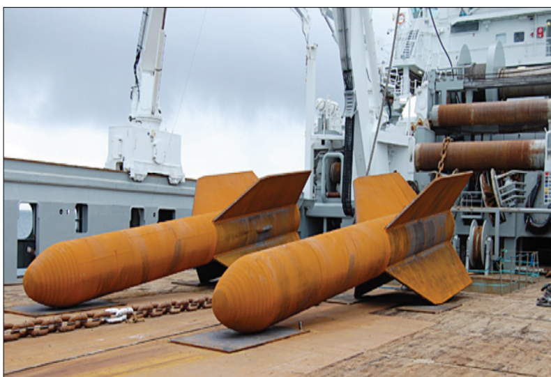
Torpedo anchors on the after deck of a large anchor handling tug
