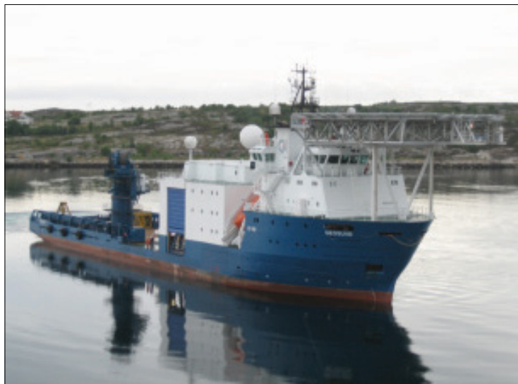
ROV support vessel (note the blue ROV hangar door)
