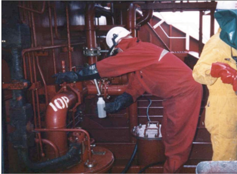
Taking samples on a chemical tanker using a sampling point. (Note the protective PPE)
