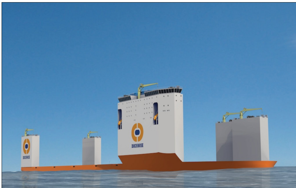
A new generation of semi-submersible heavy lift vessel the Type "O". This is an artist's impression but this vessel is under construction
