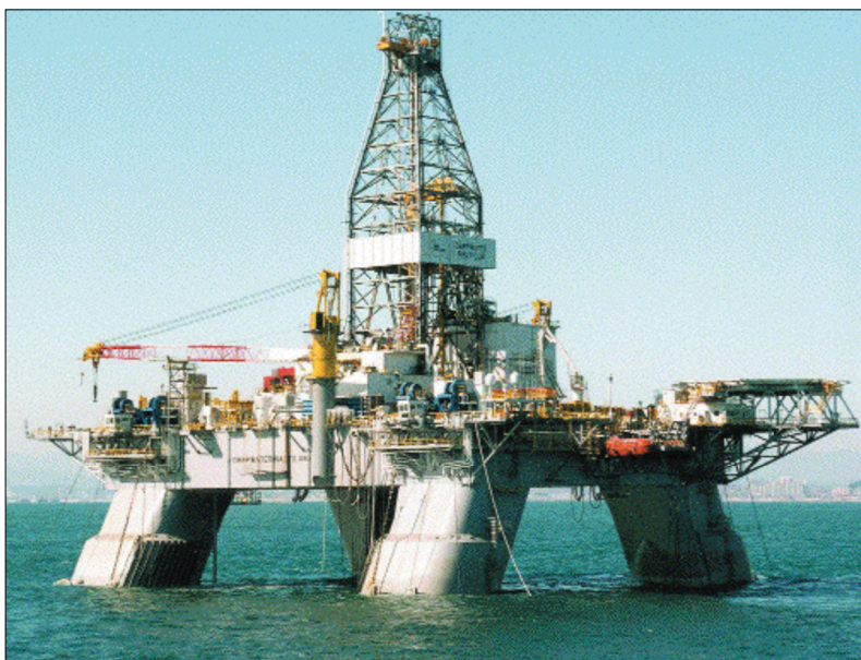
Semi-submersible Mobile Offshore Drilling Unit (note the anchor chains)
