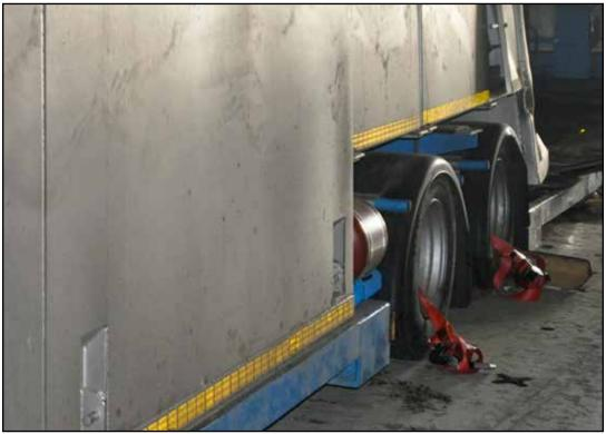
Figure 29: A 30t trailer with no securing points, secured by wheels
