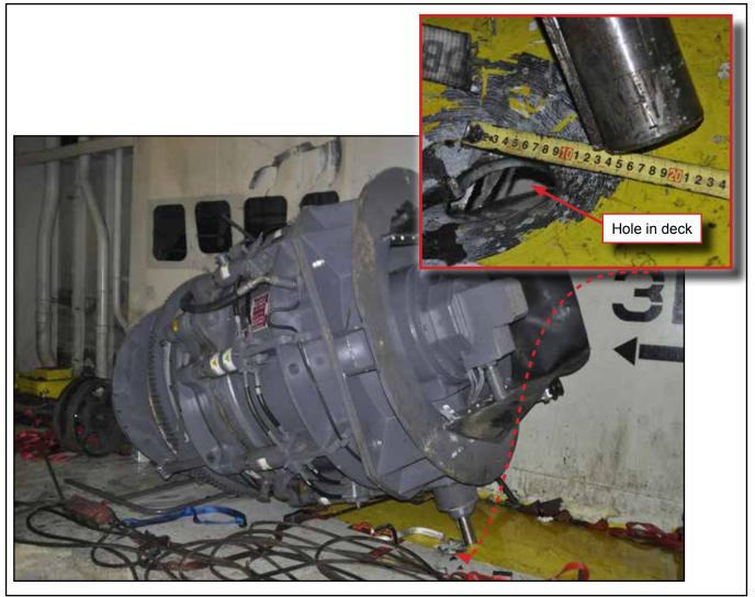
Figure 10: Component from stone crusher that fell onto deck 6
