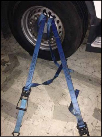
Figure 28: Lorry secured using web lash to wheels
