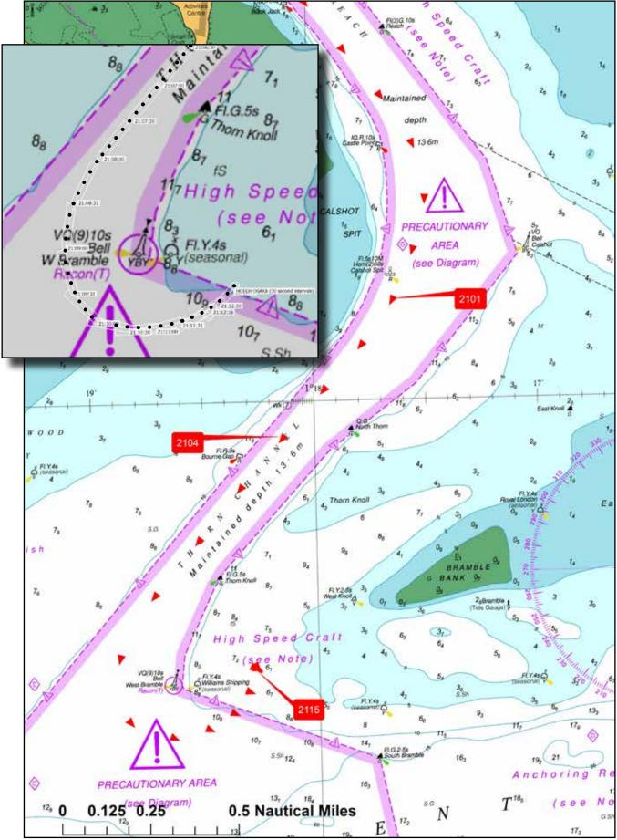
Figure 4: AIS track showing grounding position (with inset showing reconstruction of track)
