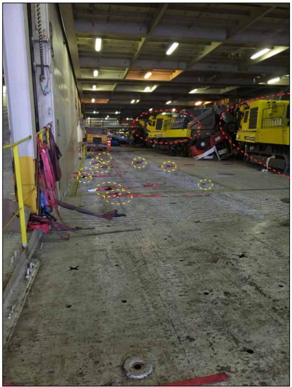
Figure 17: Original stowage position of two powercrushers, broken lashings visible on deck. Post-shift positions to starboard
