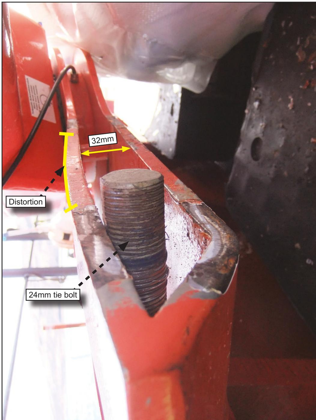
**Figure 12:** A 24mm tie bolt through a 32mm slot
