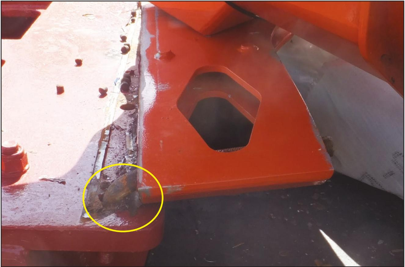
**Figure 9:** Bent tie bolt on the inboard side of the crane pedestal (circled)
