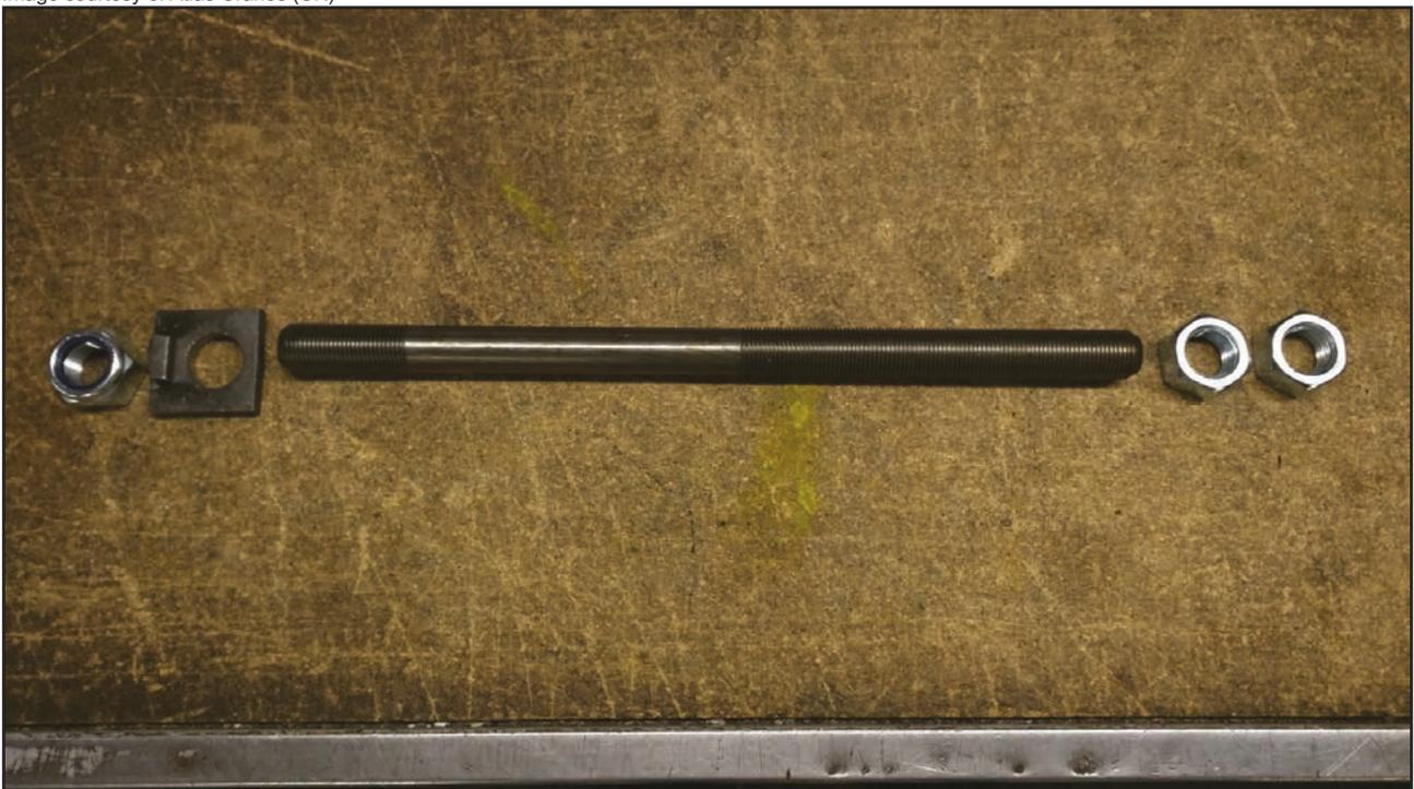
**Figure 15:** Example of an M24 tie bolt with two plain nuts, one lock nut and a tab washer
