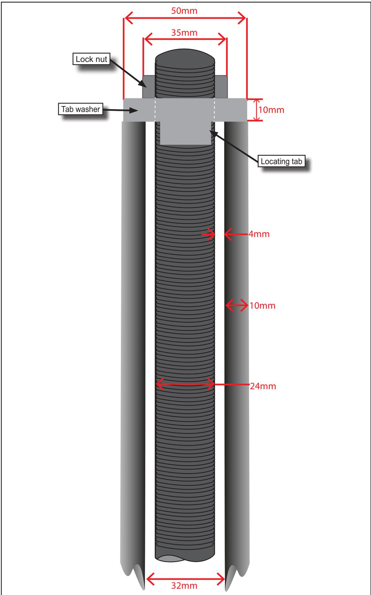
Figure 24: Diagram showing the tab washer arrangement
