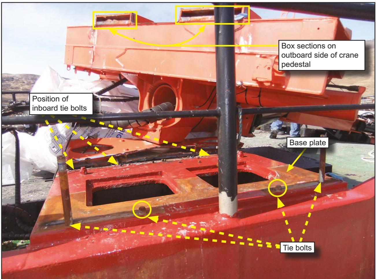
**Figure 7:** The positions of the tie bolts
