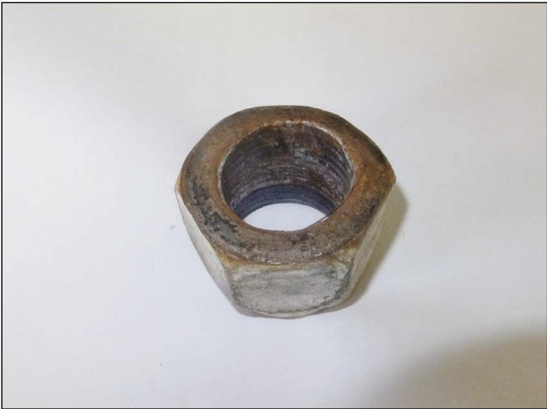
**Figure 6:** One of the failed nylon inset lock nuts
