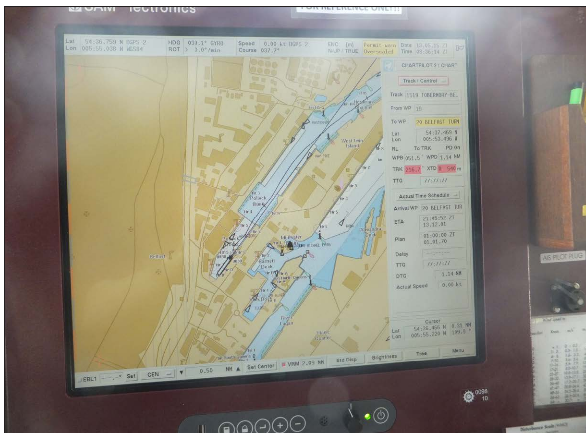
Figure 12: Hamburg's ECDIS display showing AIS information
