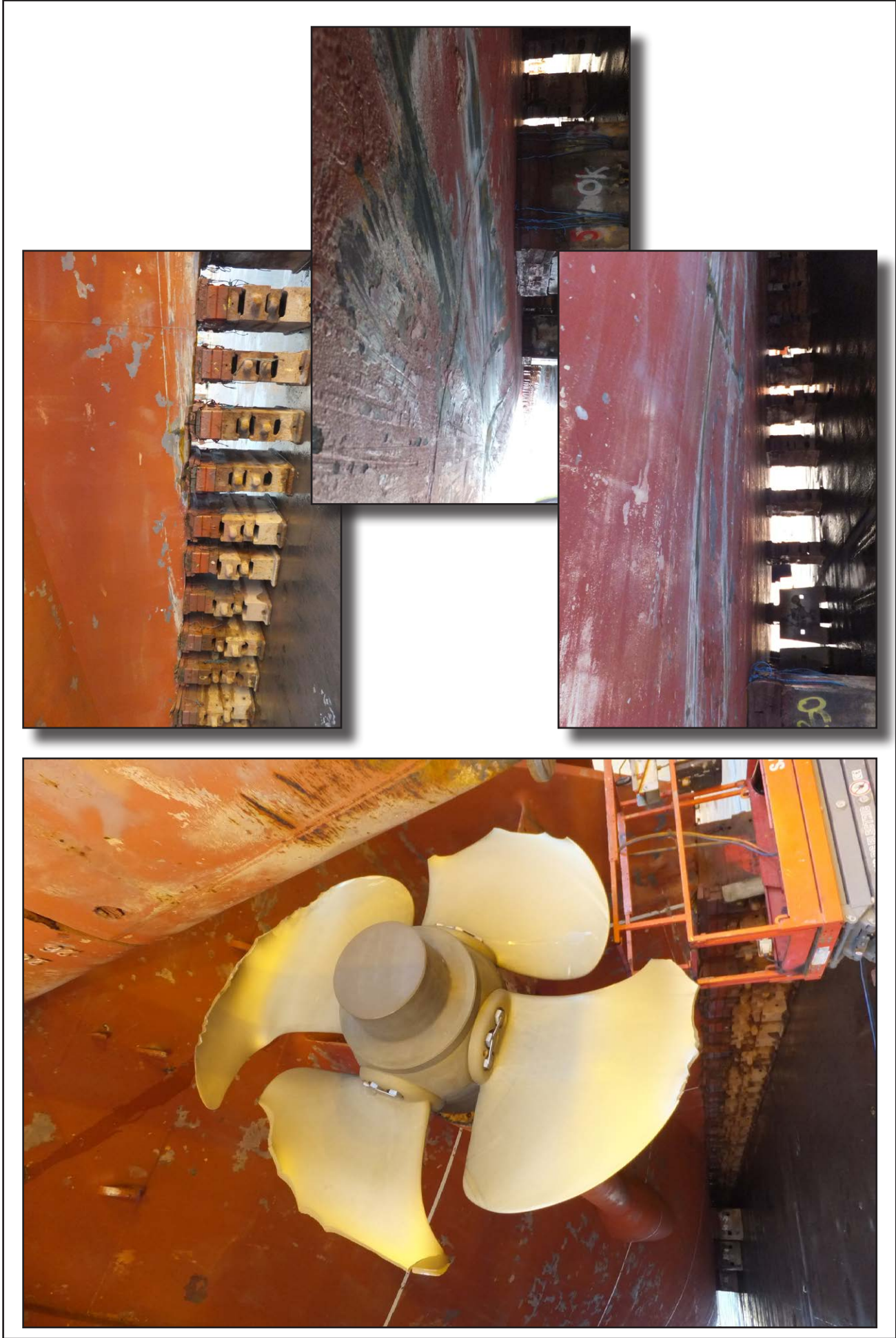
Figure 11: Photographs of hull and propeller damage
