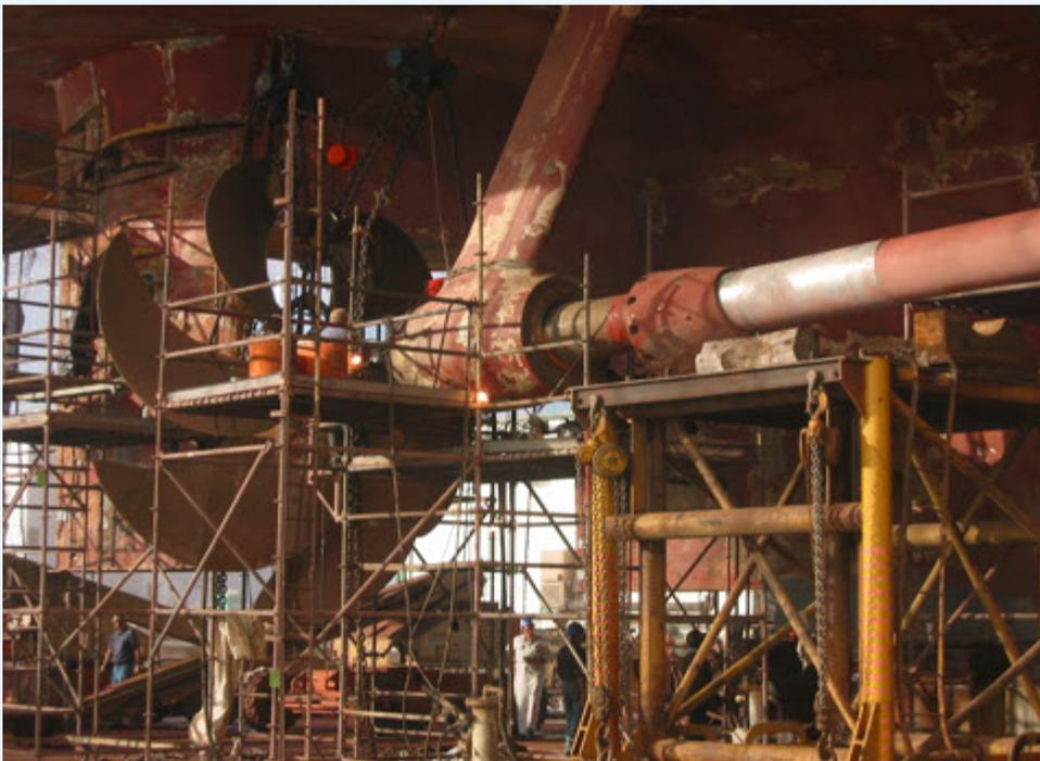
A COMPAC water-lubricated propeller shaft
