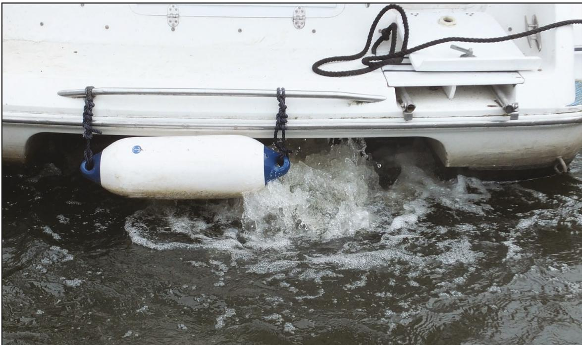
**Figure 2:** Wet exhaust at boat's stern
