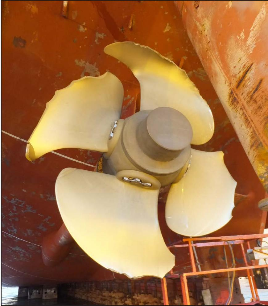
Figure 1: The damaged port propeller
