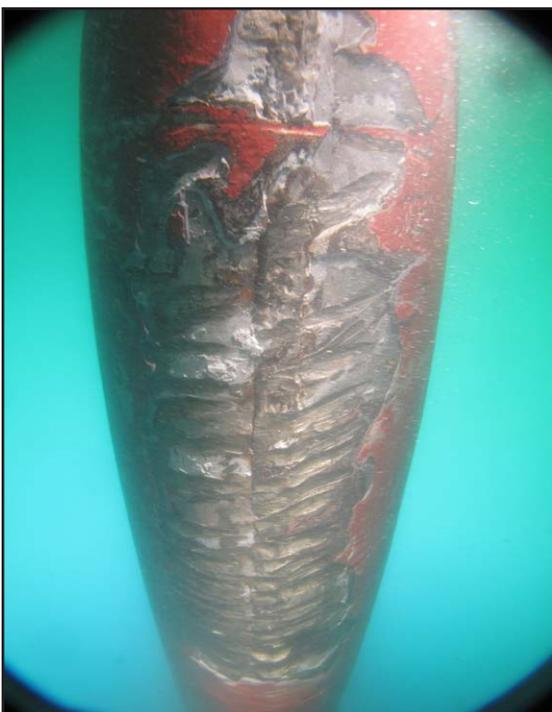
Figure 1: Damage to port rudder
