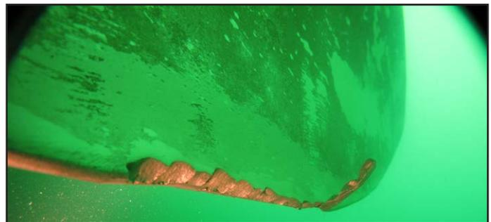
Figure 2: Damage to starboard propeller tip
