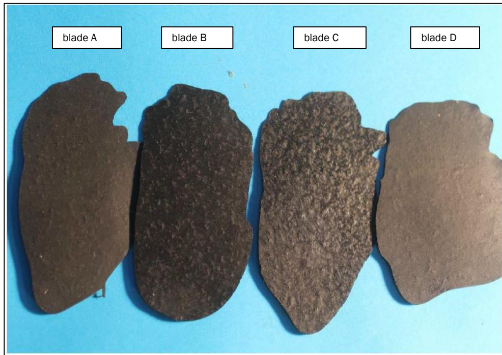
Figure 10 Surface replicas of the cavitation erosion on the blades of the starboard propeller
