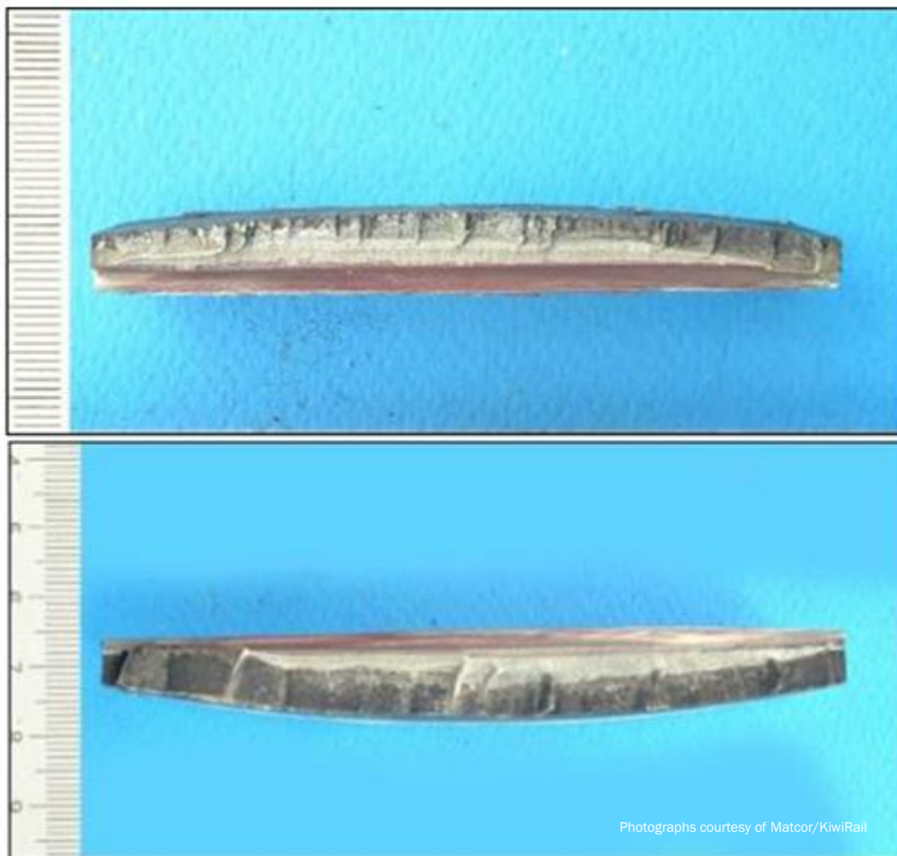
Figure 15 Fracture surfaces found on the starboard rudder stock
