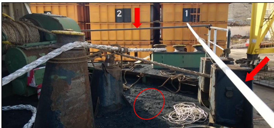
Figure 5: Temporary railing and grit on the aft mooring deck
