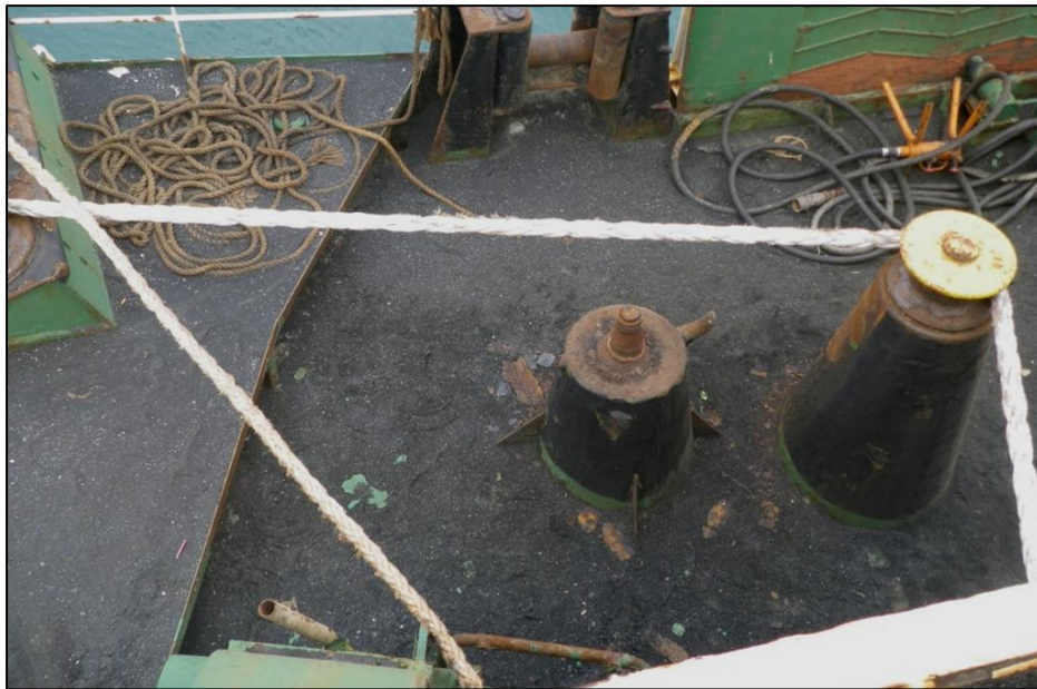
Figures 12: The two pedestal fairleads showing the different height
