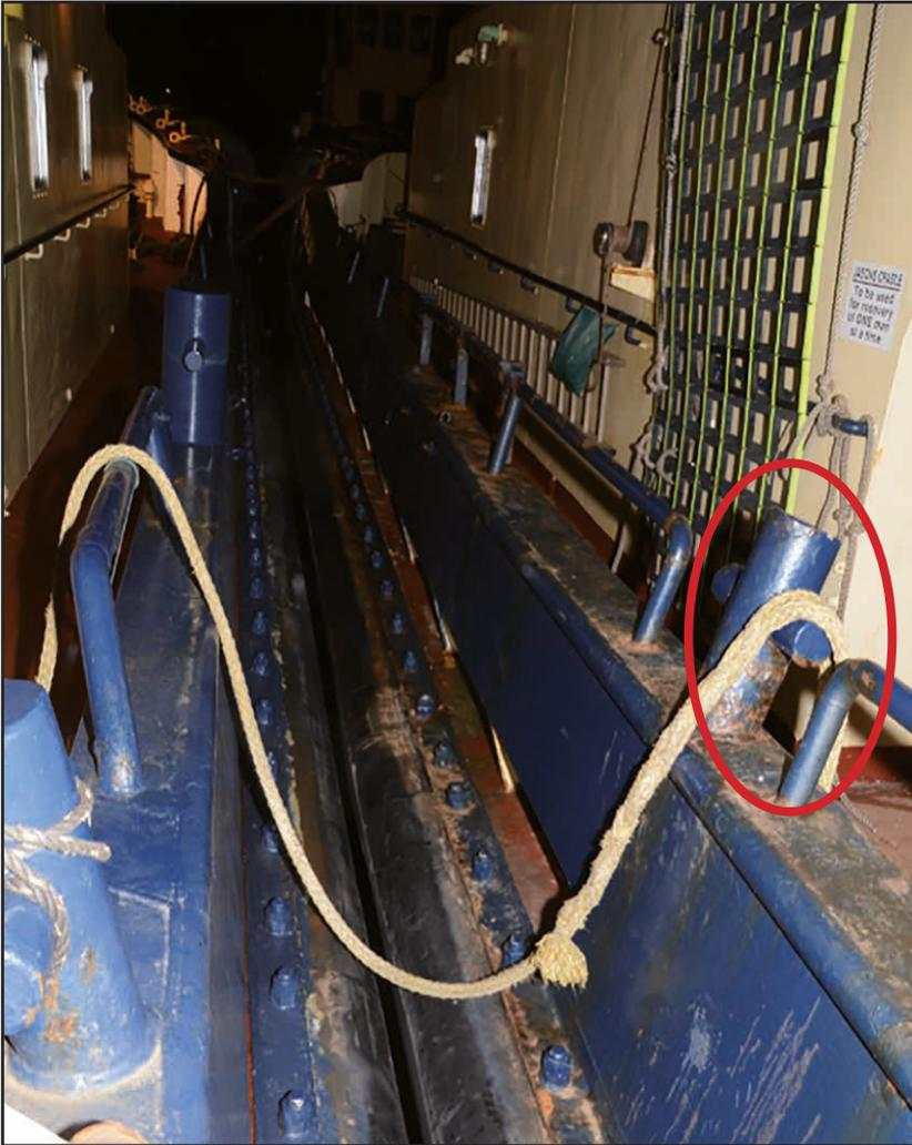
Figure 1: Reconstruction of how the amidships mooring rope was found after the accident
