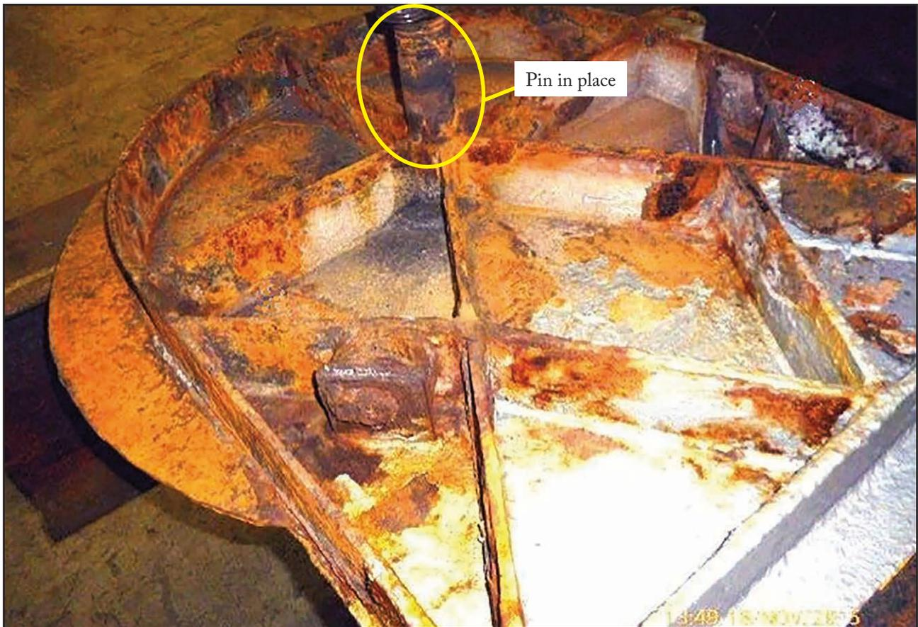
Figure 2: Port turntable (upside down) with pin in place
