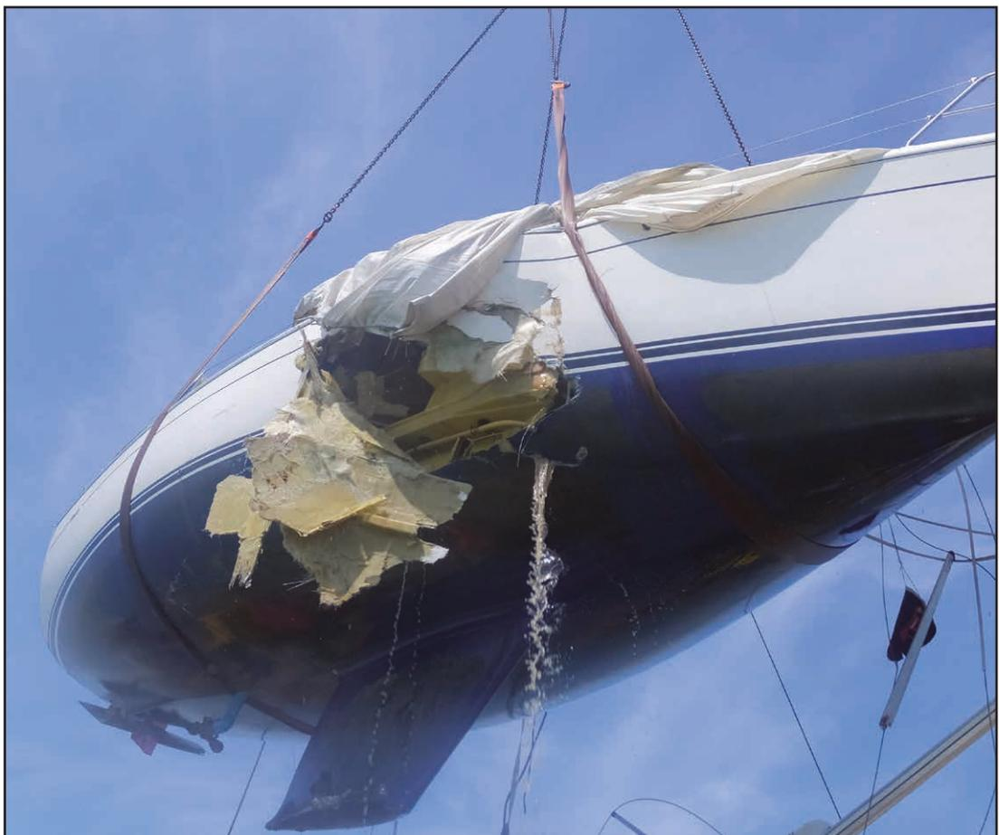
Figure 3: Damage to starboard side of yacht
