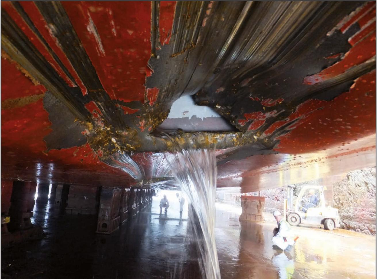
Figure 2: Hull breach and raking damage
