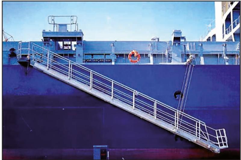
The turntable at the top of the accommodation ladder was secured to the platform with a bolted central pivot pin, and was supported by two sets of roller bearings.
