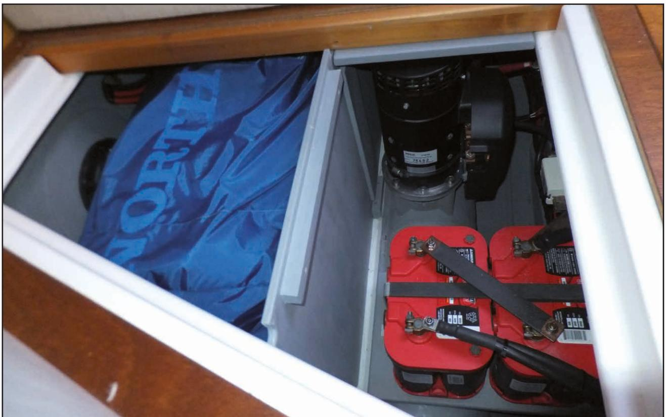
Figure 1: Typical bow thruster installation showing electric motor and dedicated batteries
