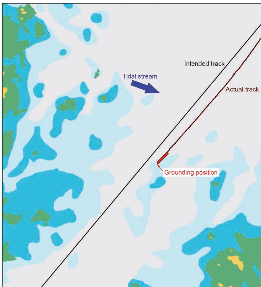
Figure 1: Chart showing the vessel's intended and actual tracks
