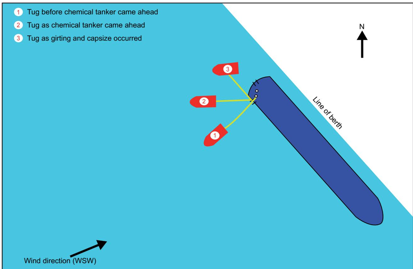
Figure: Indicative relative movement of the mooring launch
