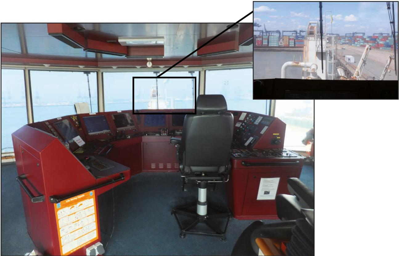
Figure 2: Bridge conning position (inset: obstruction)
