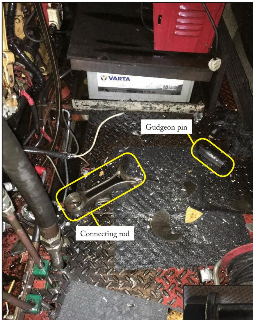
Figure 2: Connecting rod, piston and gudgeon pin ejected from the engine (inset: failed bottom end bearing bolt)
