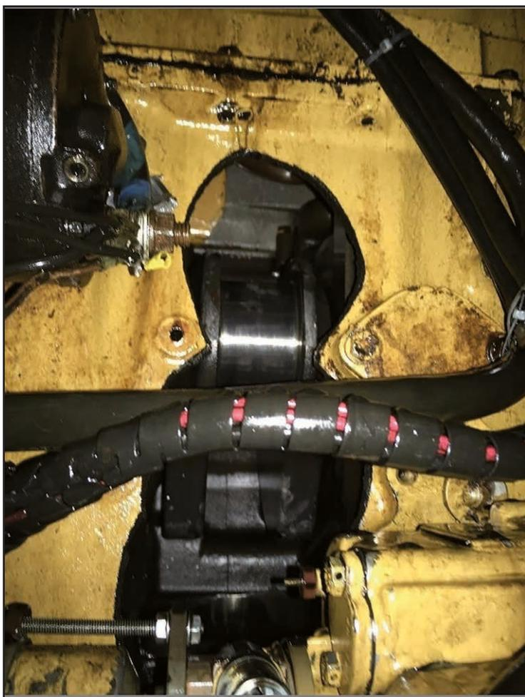
Figure 1: Crankcase damage caused by connecting rod/piston assembly
