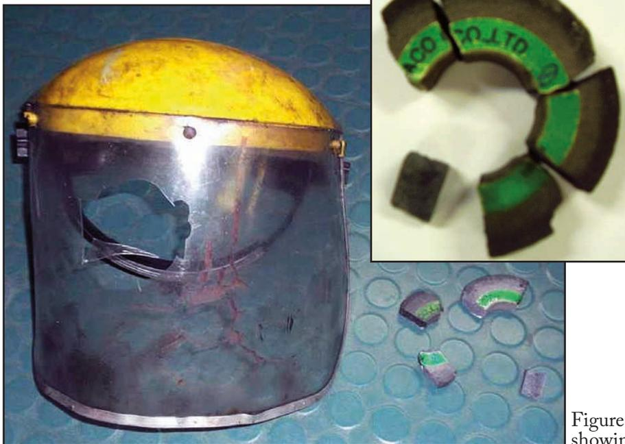
The crew could not determine the speed rating of the exploded grinding disc as there were no more similar discs on board. It was most likely to have been rated well below 22000rpm as most general purpose grinding discs are rated between 5000 and 15000rpm.
