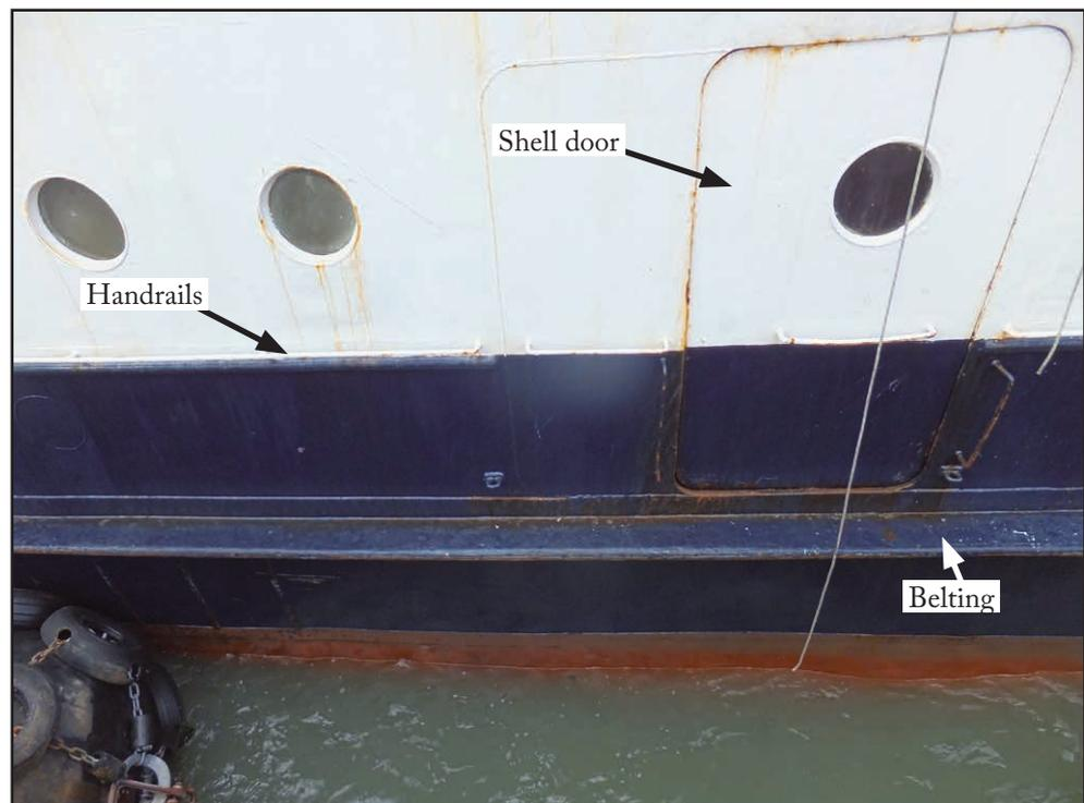
Figure 1: Shell door, ship's side belting and handrails
