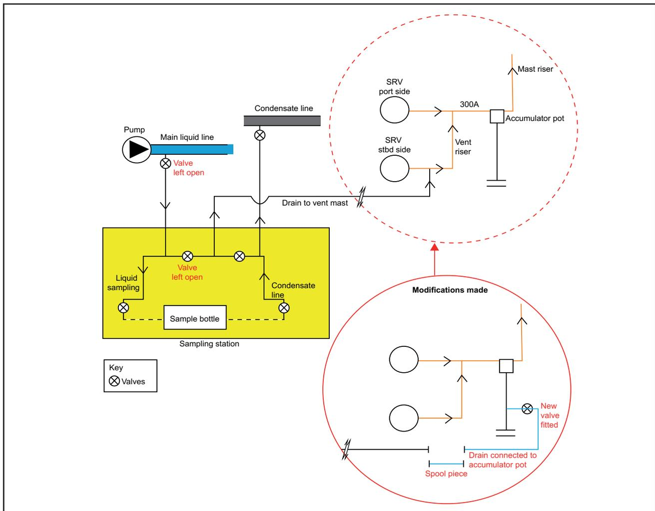
Figure: Before and after modification
