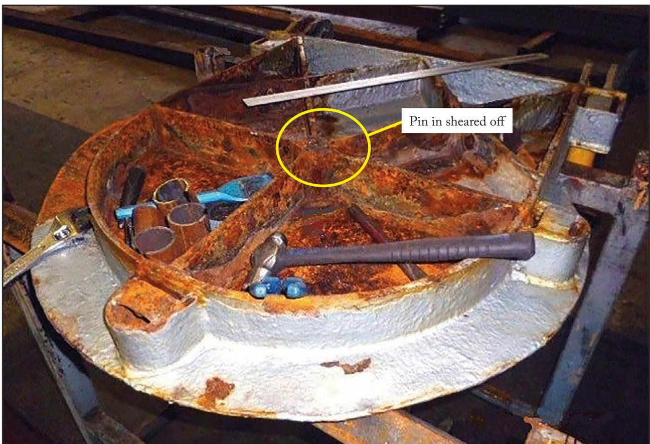
Figure 3: Starboard turntable (upside down) with pin sheared off
