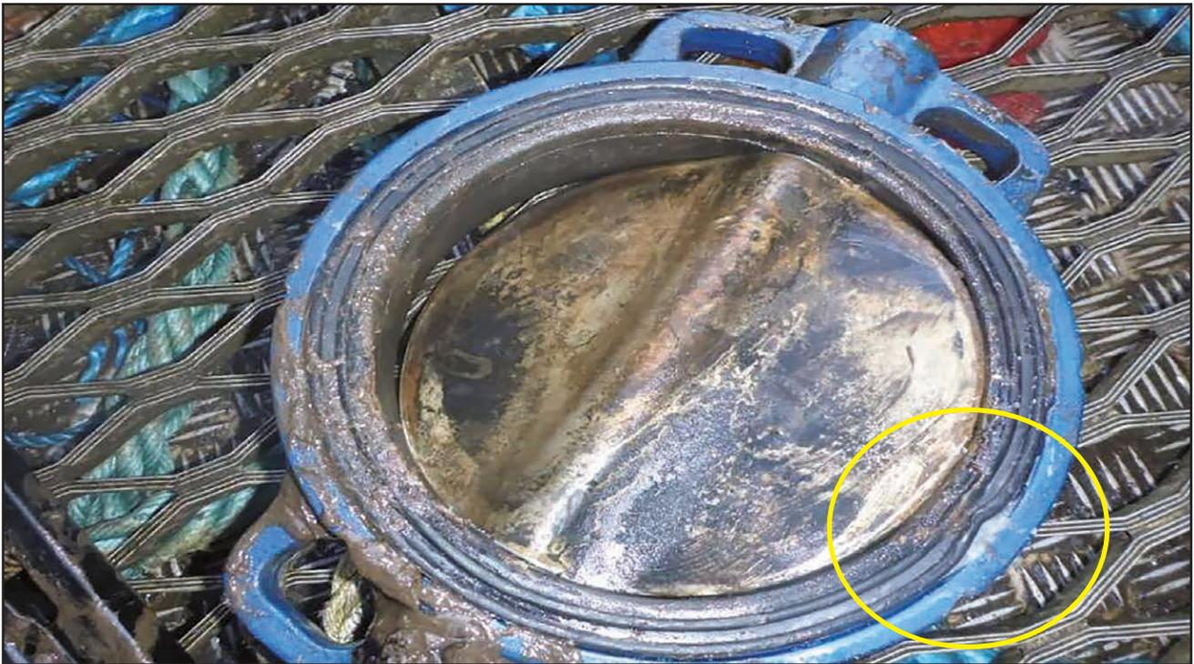
Figure 2: Defective butterfly valve
