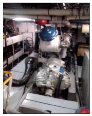
Figure 4: Restricted accessibility around the port main engine
