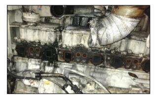
Figure 3: Dismantled exhaust manifold, turbocharger and exposed exhaust ports
