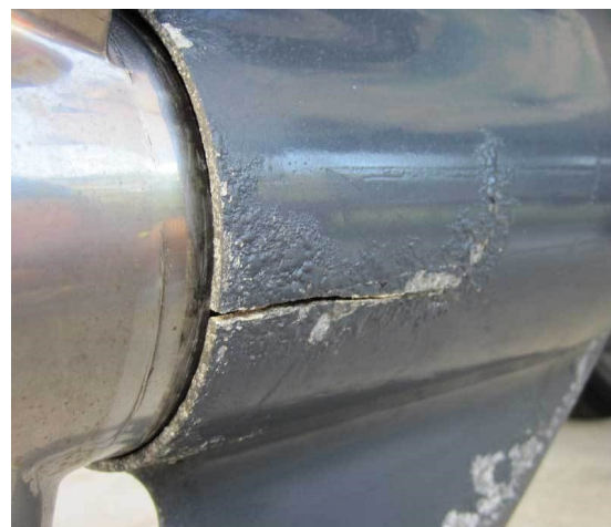
Cracked prop. housing
