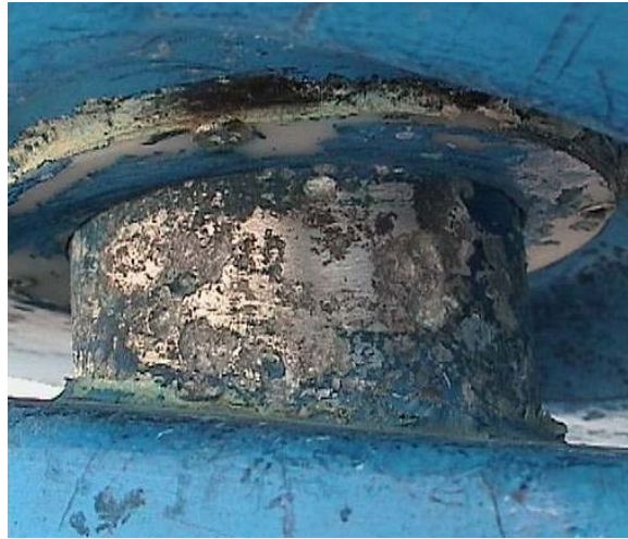
Corroding rudder stock, caused by electrical connection to prop. shaft
