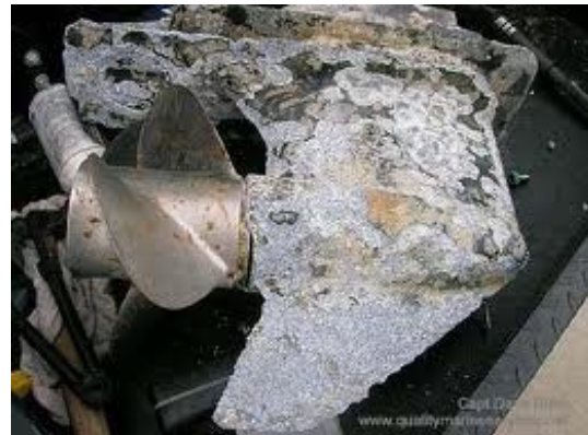
Corrosion of Aluminium in sail drive coupled with Stainless Steel
