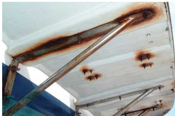
Corrosion of swim platform support brackets
