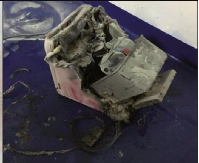
Figure 1: Similar travel fridge to the one in the cabin      Figure 2: Remains of the fridge after the fire
