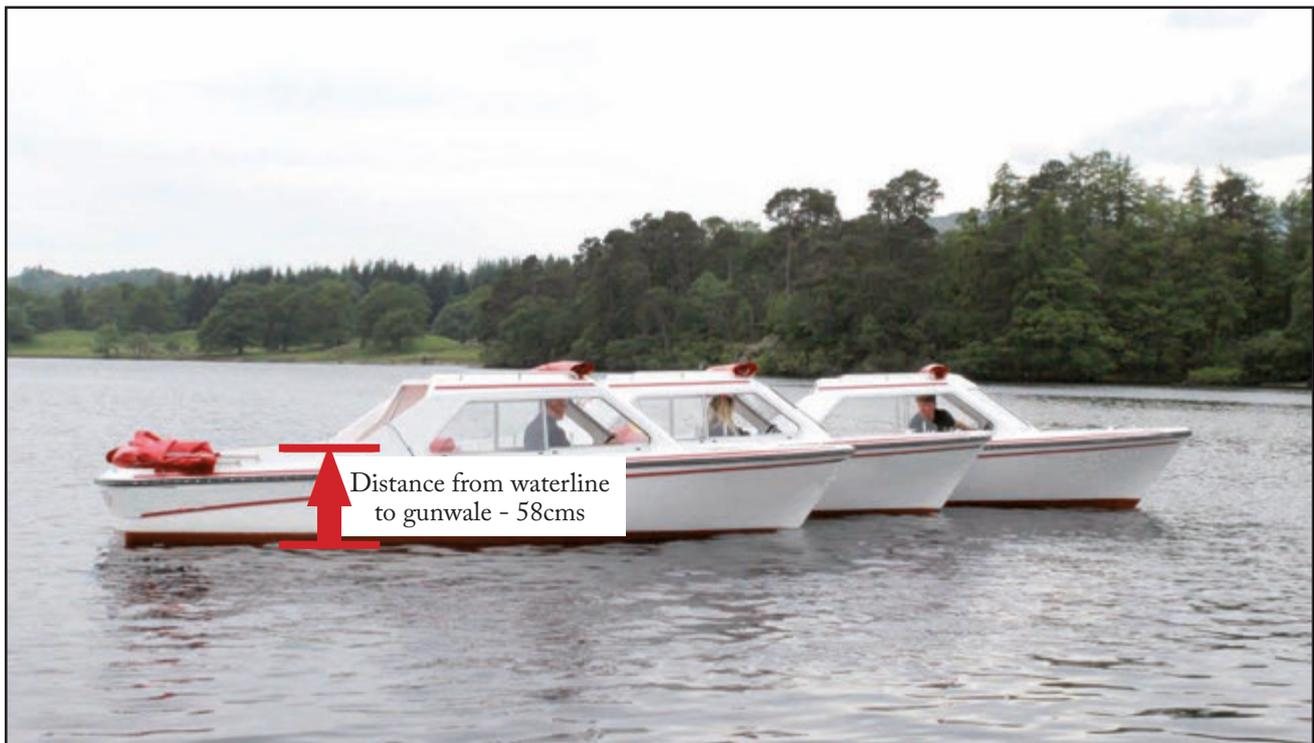
Figure 1: Small self-drive motor boats
