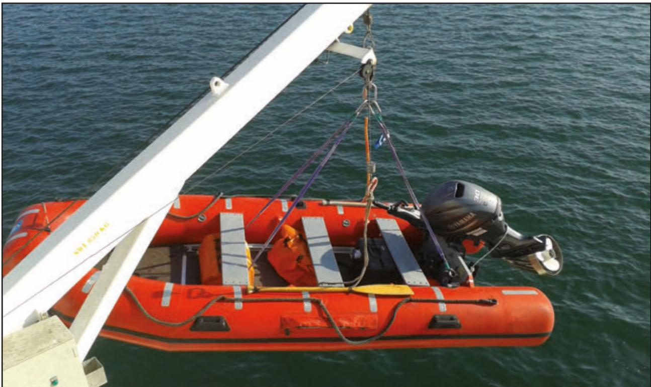
Figure 2: Lifting strops correctly fitted to inflatable rescue boat
