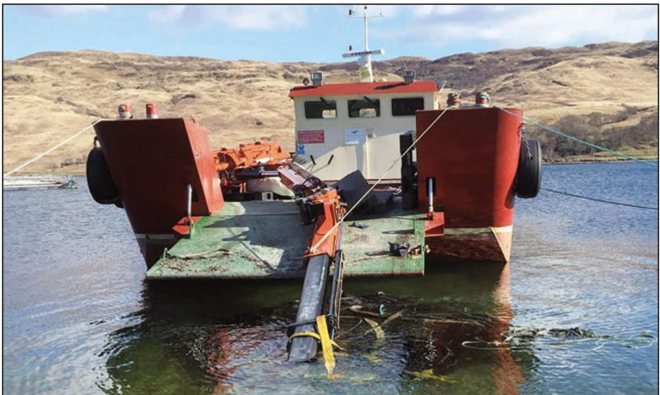
Figure 1: Collapsed crane
