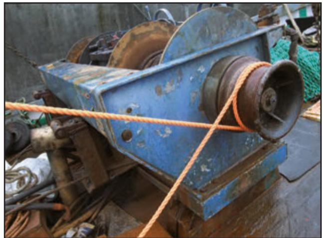
Starboard whipping drum with 1.5 turns of rope
