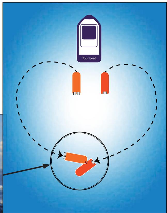
Figure 1: Power turn manoeuvre and collision
