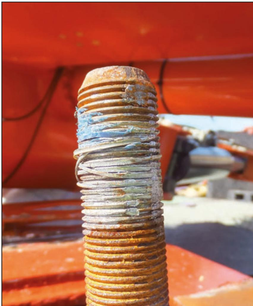
Figures 2 and 3: Failed nut and tie bolt
