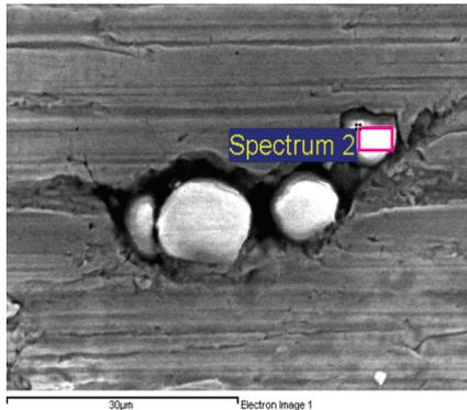
Different sized particles can create different risks with the potential to cause damage at different locations in the fuel system. For example, particles can be small enough to pass through fuel pump barrel/plunger clearances, or large enough not to enter those same clearances. In either case, they will not cause abrasion at the fuel pump barrels/plungers, whereas those of a size comparable to the relevant clearances would be expected to cause damage in way of the fuel pumps.
