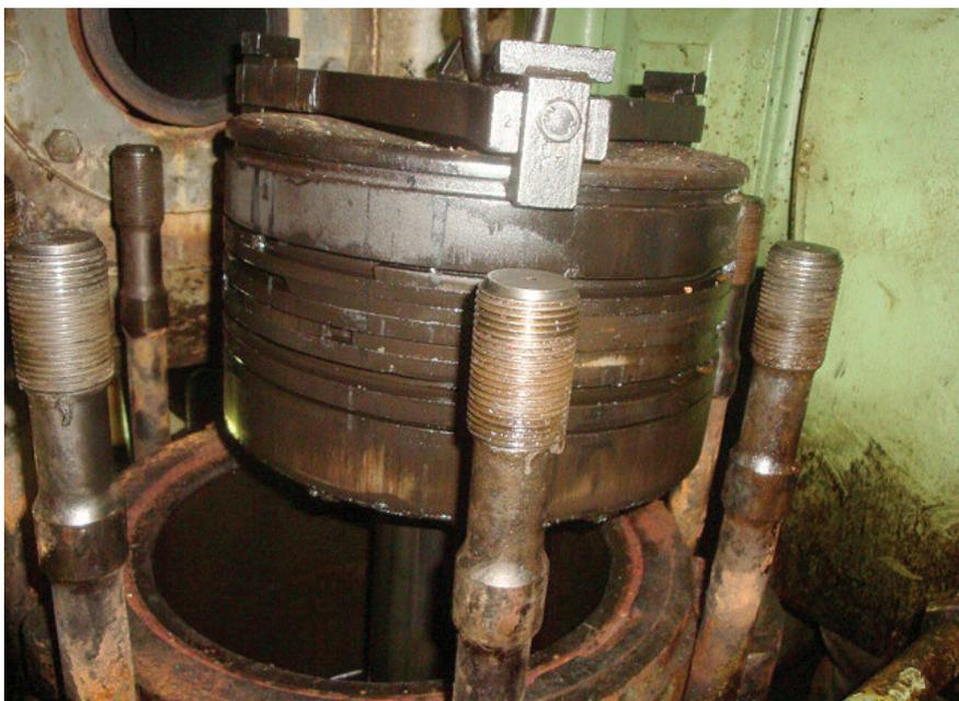
Refinery catalytic fines in marine fuel oil are not a new problem but in recent years there appears to have been an increase in the frequency of engine damage caused by these highly abrasive particles.
