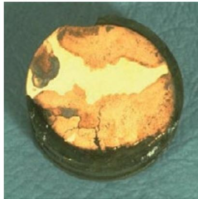
Figure 4 - Dezincification in 60-40 brass valve stem
