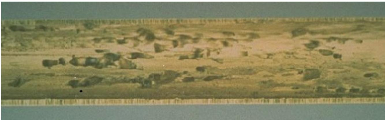
Figure 3 - Erosion corrosion of 90-10 copper-nickel when exposed to excessive flow rates
