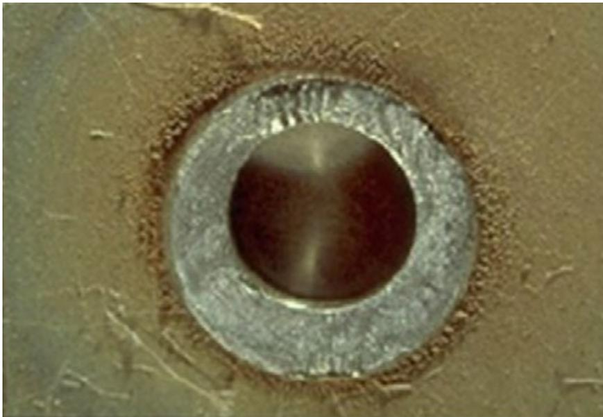
Figure 2 - Crevice corrosion under a washer on 316 stainless steel immersed in sea water for 3 months
