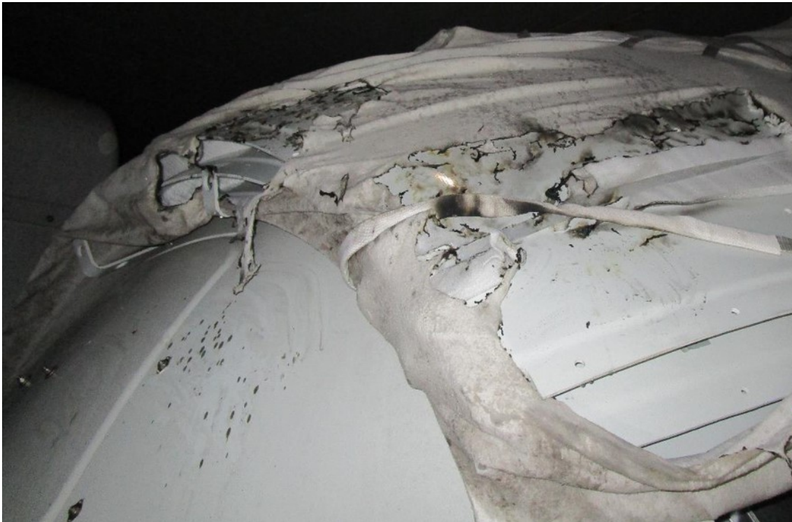
Figure 4: Cargo covering material and cargo surface damage
