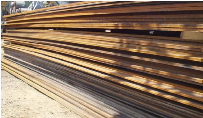
Steel plates stored outside exposed to the elements
