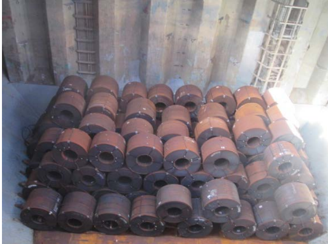
Rusted cargo of coils in a ships hold
