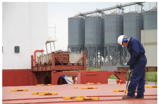
Ultrasonic hatch cover testing
