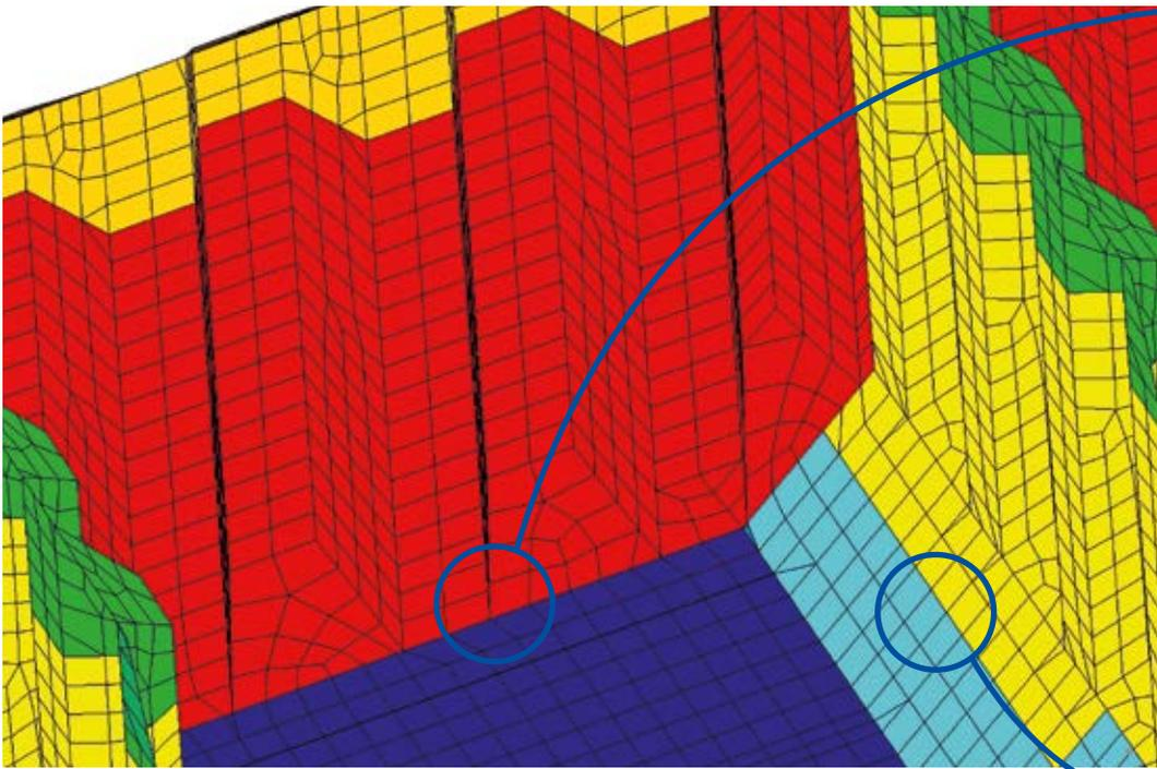
Feasibility study of product/chemical tanker. Cargo hold model with very fine mesh models of the hinges.
