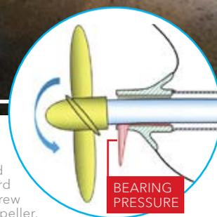
Most of the reported damages have been observed on the aft-most part of the aft bearing and were accompanied by high bearing temperatures with an abrupt rate of rise. Expensive and time-consuming repairs were the consequences.
