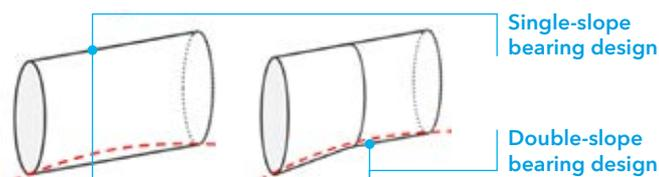
Multi-sloped bearing improves the contact area: the coloured plot reflects the extent of the gap between the shaft and the bearing.
