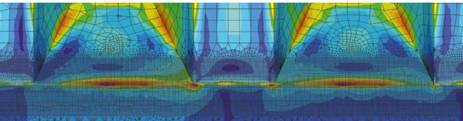
Feasibility study of product/chemical tanker. Maximum surface stresses (for hotspot stress assessment) at lower hinge of transverse bulkhead (see high stress concentration in way of inclined plate corner located close to a diaphragm web plate in lower stool).
