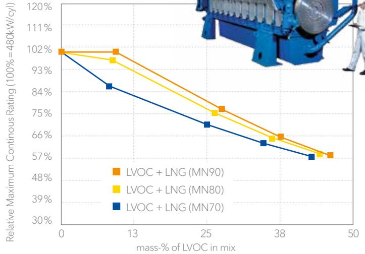
Relative maximum continuous rating in relation to LVOC mass ratio in per cent in LNG mixes.
