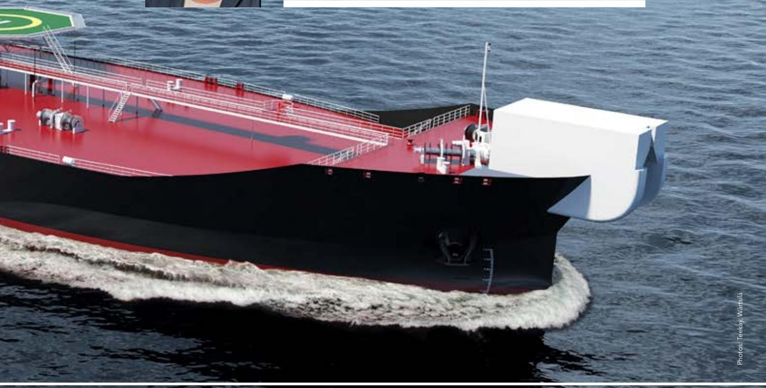
> Since more than 50 per cent of Norway's VOC emissions occur during storage and loading of crude oil, stringent emission reduction regulations have been implemented which apply to all shuttle tankers receiving crude oil from offshore processing platforms on the Norwegian continental shelf. VOCs evaporating from the cargo tanks during loading must be captured by a VOC recovery plant.
