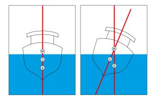
Figure 4: Diagrams to illustrate Centre of Gravity and Buoyancy, Metacentric height and Metacentre
