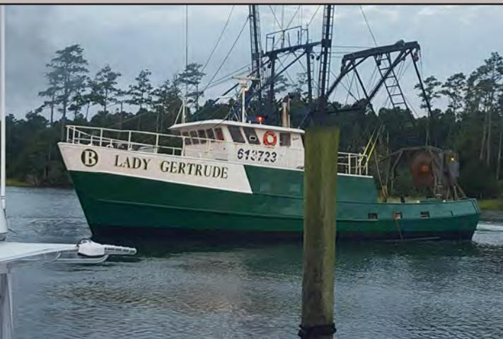
**O**n August 15, 2016, about 0150 local time, the fishing vessel *Lady Gertrude* began flooding through its propulsion shaft stern tube while preparing to dredge for scallops. The crewmembers abandoned ship and were rescued by a good Samaritan vessel before Coast Guard search-and-rescue assets arrived. The vessel sank at 0453. No one was injured. A light oil sheen was observed. The *Lady Gertrude* was valued at \$400,000.
