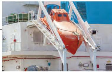
Figure 71: Exemplar enclosed freefall lifeboat in launch position on a slipway
