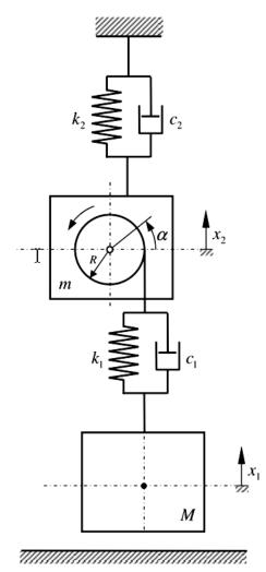
Figure 4: Schematic diagram of loading during lifting/lowering motion
