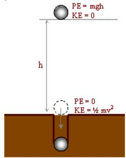
Figure 5: Diagram showing the impact force from a free falling object [4]
