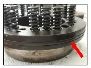
Figure 11: Oil seal fitted on the high pressure hydraulic actuating system
