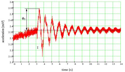
Figure 3: An example of a typical dynamic overload due to stoppage of lifting motion
