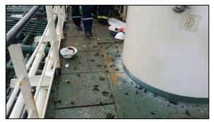
Figure 2: Parts of the slewing bearing following the collapse
