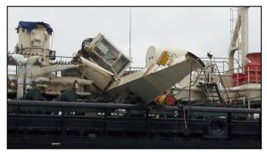
Figure 1: The collapsed deck slewing crane
