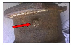
Figure 7: Plugged tell-tale (after cleaning of the brake housing)
