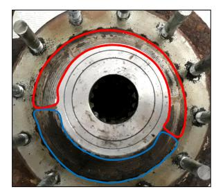
Figure 12: Uneven pressure marks on the innermost outer lamella friction surface
